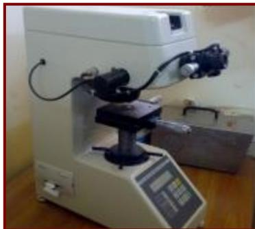
**Figure 1: Model HVS-100 Digital microhardness tester with a Vickers diamond indenter.**
