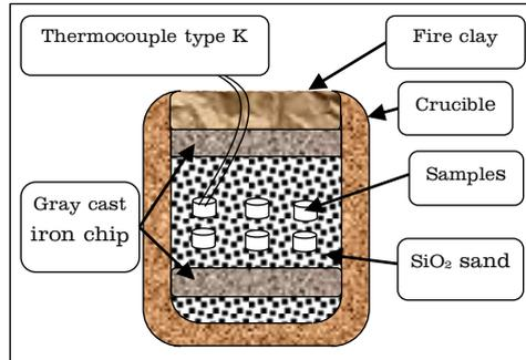
Figure (2) : sintering configuration.
