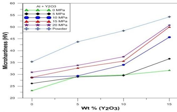
Figure (3) : effect of Y<sub>2</sub>O<sub>3</sub> on Vickers microhardness of Al- Y<sub>2</sub>O<sub>3</sub> composites
