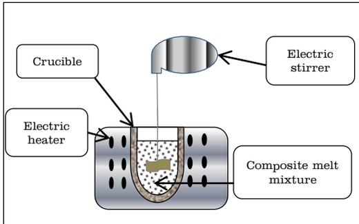
Figure (1) : stir mixer components.
