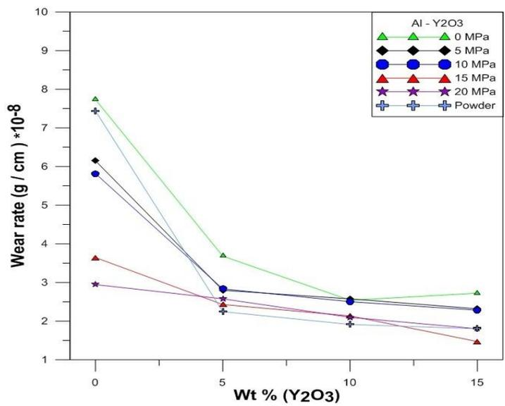
Figure (8) : effect of  $Y_2O_3$  on wear rate of Al- $Y_2O_3$  composites.
