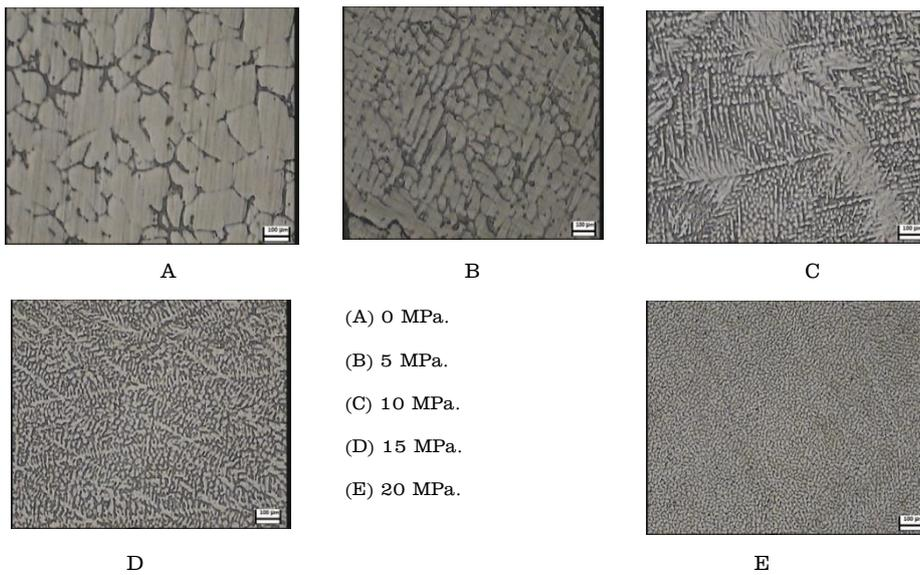
Figure (4) : microstructure of Al-5%Y<sub>2</sub>O<sub>3</sub> prepared by squeeze casting.
