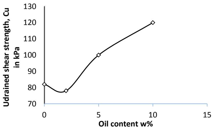
Figure 5: Undrained shear strength of soil A from vane shear test at different contamination percentage
