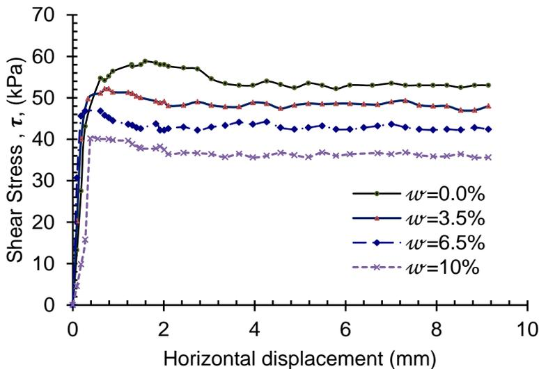
Figure 6: Relationship between shear stress versus horizontal displacement at  $(\sigma_n) = 100$  kPa
