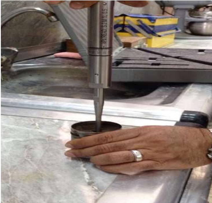
Figure 3: Hand vane shear tester
