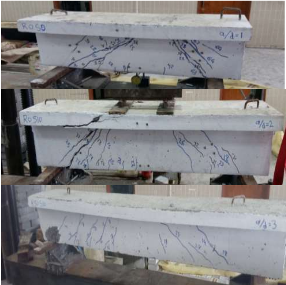
Figure (2): crack pattern for T-beams.
