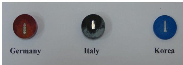
Figure (1): Three types of Dental Implant after cutting, grinding and polishing process
