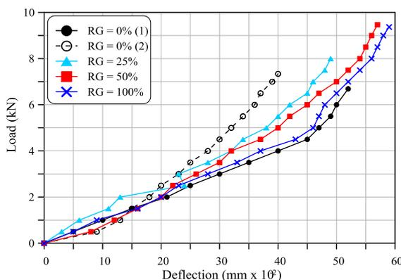
Fig. 5. Load-deflection curves for different recycled glass (RG) replacement ratios
