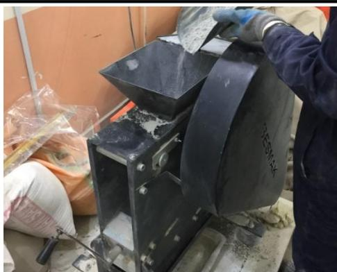
Fig. 1. Second stage crushing of the recycled glass
