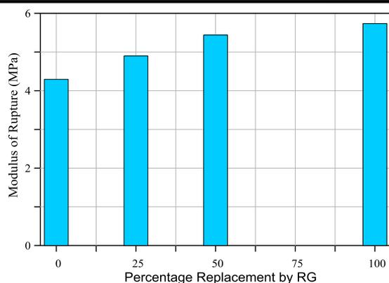
Fig. 4. Effect of replacement of silica sand by recycled glass (RG) on modulus of rupture
