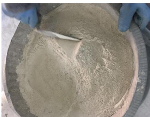
Fig. 2. The used recycled glass after crushing
