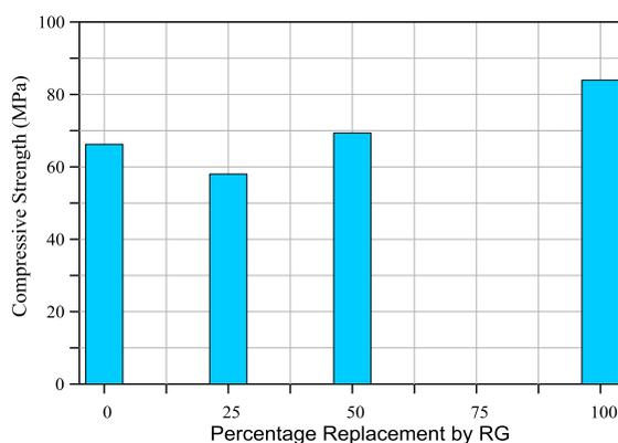
Fig. 3. Effect of replacement of silica sand by recycled glass (RG) on compressive strength
