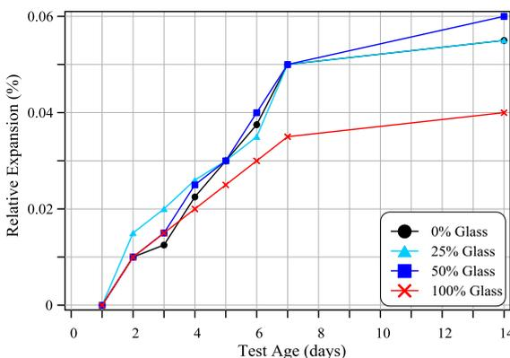
Fig. 6. Percentage relative expansion for different recycled glass (RG) replacement ratios
