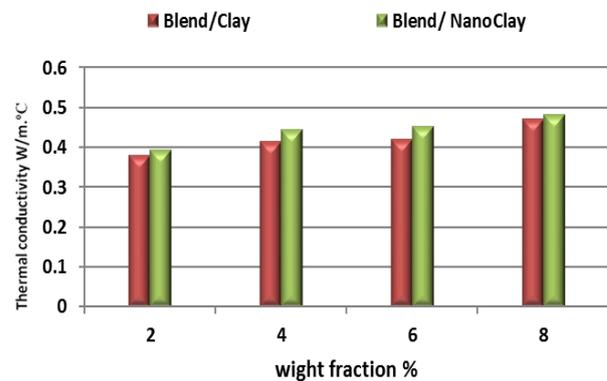
Figure 3: The Thermal Connectivity value relation with weight fraction for particles and nano (Clay + Blend) exposure to UV.
