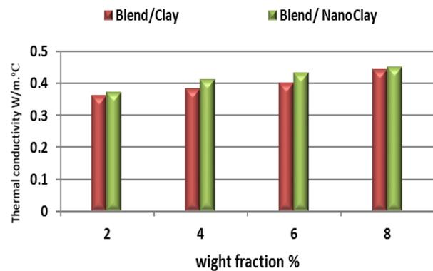
Figure 2: The Thermal Connectivity value relation with weight fraction for particles and nano (Clay + Blend) at natural condition.
