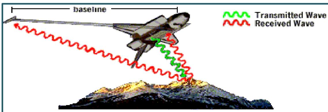
Figure(1) SRTM Single-Pass InSAR Configuration ( Bamler, 1999).
