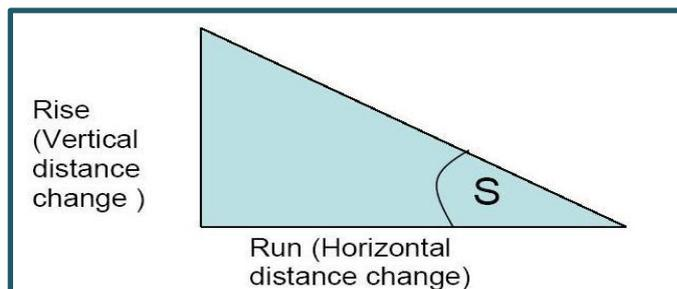
Figure (4) Definition of slope as the angle from horizontal.
