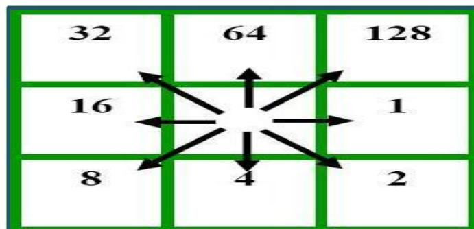
Figure (5) ESRI Flow direction encoding.
