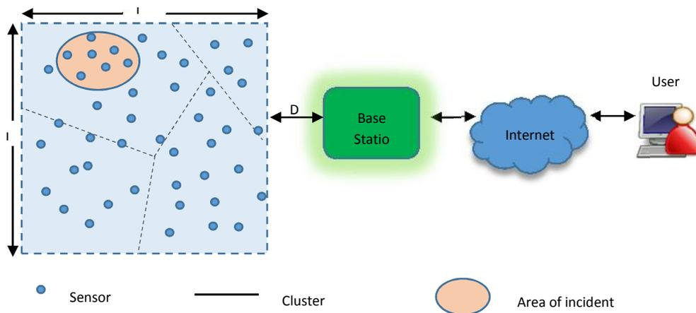
Figure 1. Wireless Sensor Network
