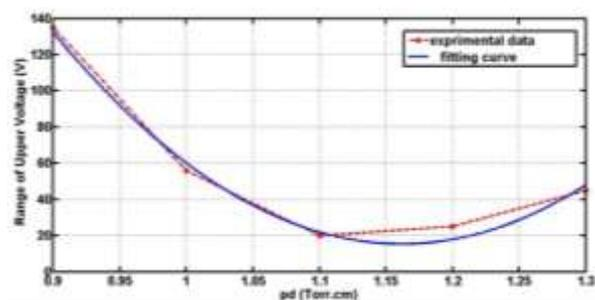
Figure 3. The range of upper voltage of glow discharge of air as a function of working pressure with fitting curve
