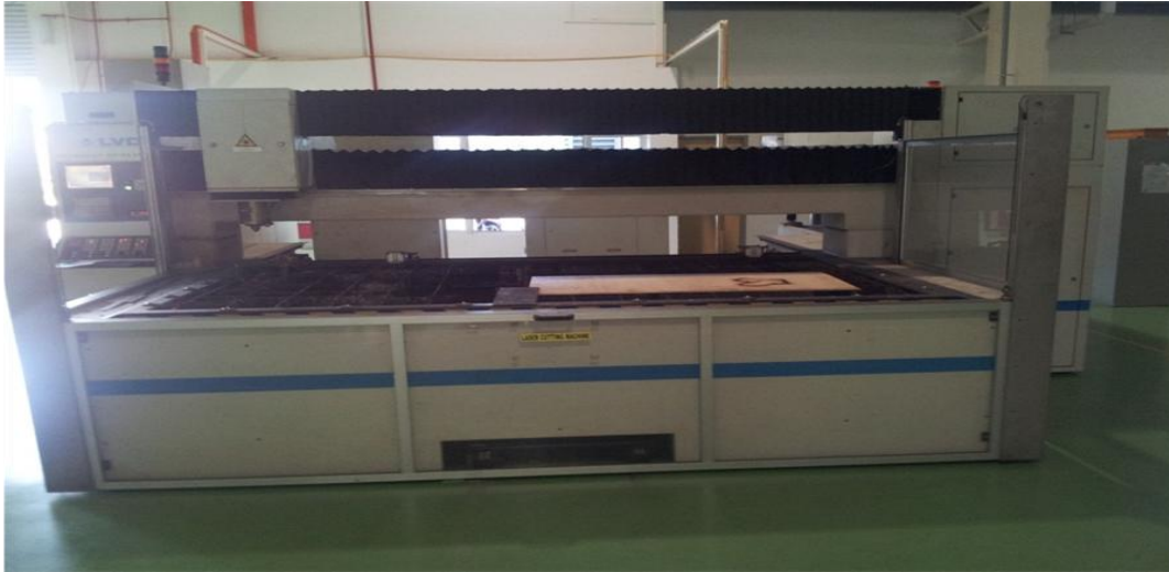
Figure 2. A laser cutting machine LVD Model 2513 with a maximum output power of 4000 Watt, 6301 \mu\text{m} wavelength, available in University technical Malaysia (UTeM).
