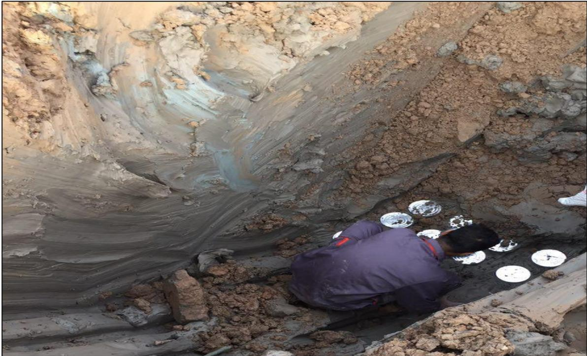
**Plate 1.** Undisturbed soil samples from an open bit.
