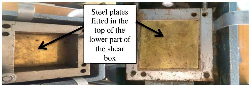
**Plate 2.** Steel plate fitted on the top of the lower part of the shear box.
