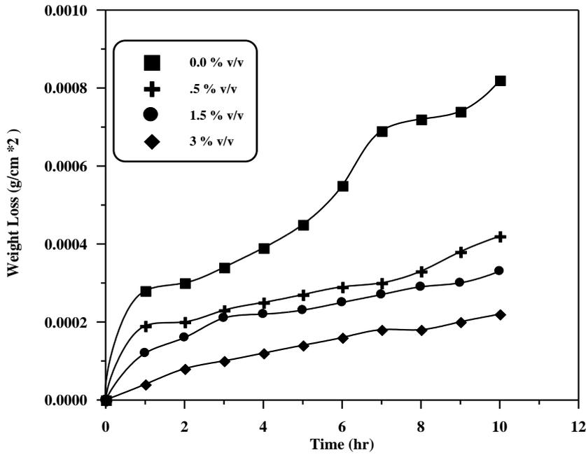
**Fig. 2: Variation of weight loss with time for brass in 1M HCl solution containing different concentrations of tobacco extracts.**
