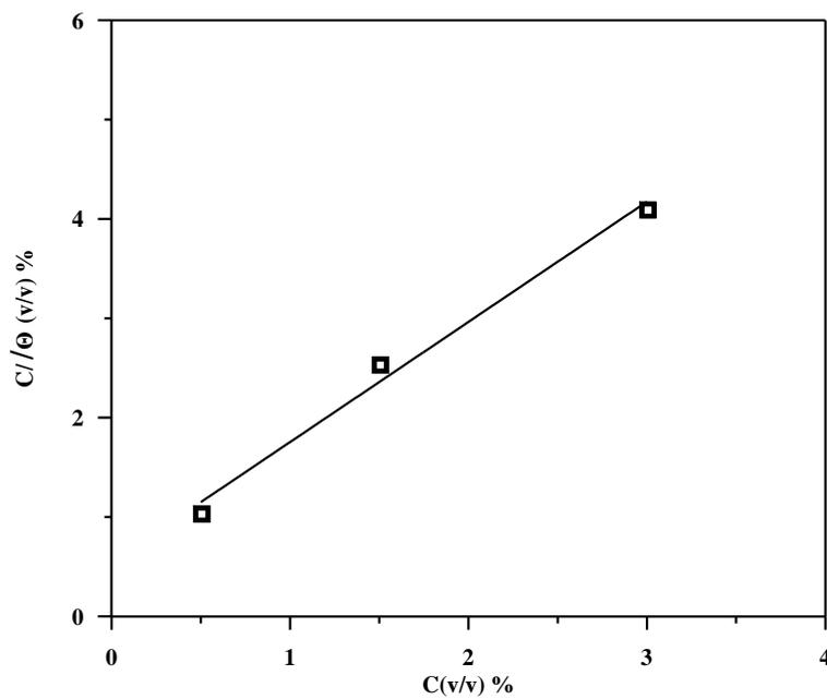
**Fig.9: Langmuir isotherm plots for the adsorption of tobacco extracts on the surface of brass in 1M HNO<sub>3</sub>**
