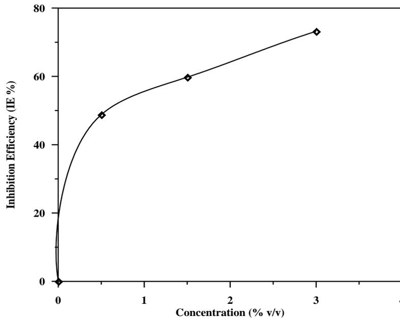
**Fig 5: Variation of inhibition efficiency with concentration in 1M HNO<sub>3</sub> solution.**
