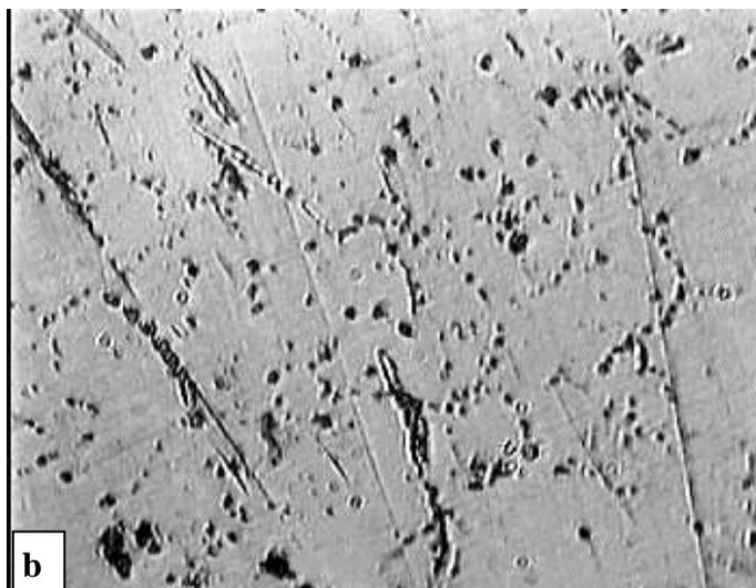
**Fig.7: L.O.M. images of brass immersed in HNO<sub>3</sub> solutions (a = 1M HNO<sub>3</sub>, b = 1M HNO<sub>3</sub>+3% tobacco extracts for ten hrs. (Magnification 400X).**
