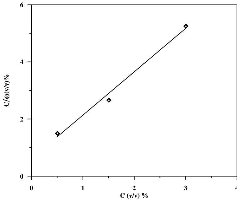
**Fig.8: Langmuir isotherm plots for the adsorption of tobacco extracts on the surface of brass in 1M HCL.**
