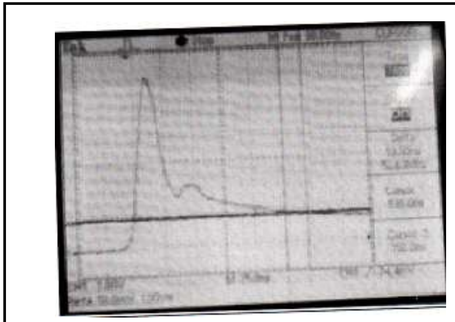
Fig.(8)The laser pulse duration received by photo detector
