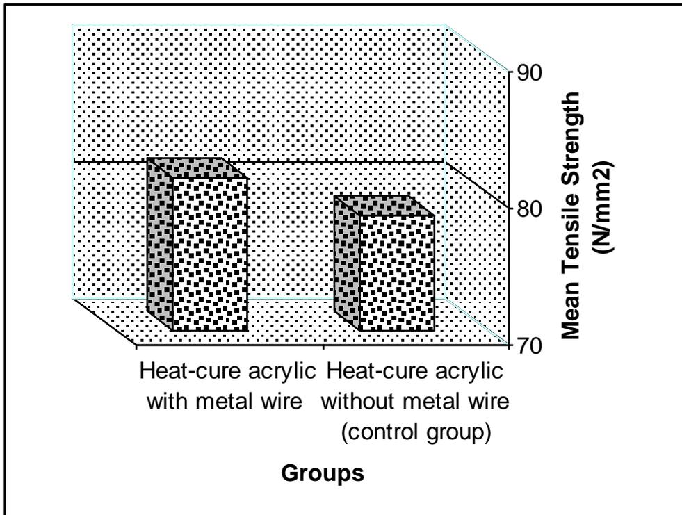
Figure3: Bar chart show the mean values for tensile strength (N/mm<sup>2</sup>) of heat-cure acrylic resin denture base as influenced by metal wire.
