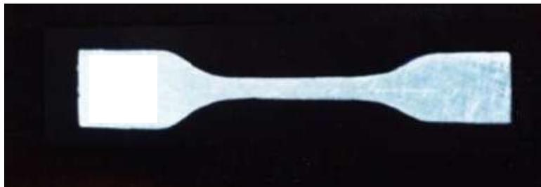
**Figure (1): -Metal pattern for tensile bond strength.**
