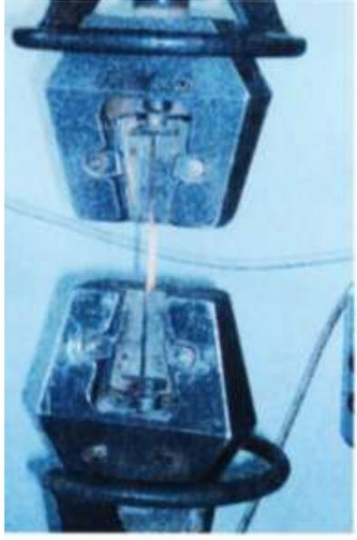
**Figure (2): Specimen under tensile bond strength test.**
