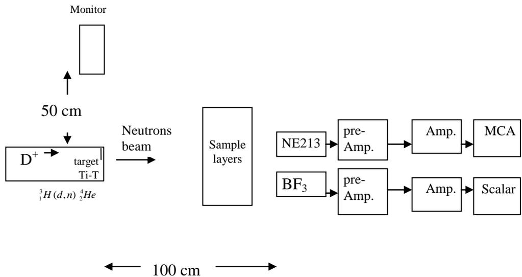
Fig. 1. Geometrical arrangement of the experimental measurements
