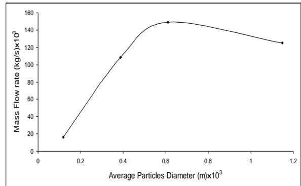
Fig. 9. Effect the Particles Sizes on the Flow (Without Lubricants)
