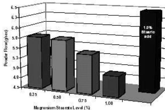
Fig.2. Effect Stearic Acid on Powder Flowability [8]
