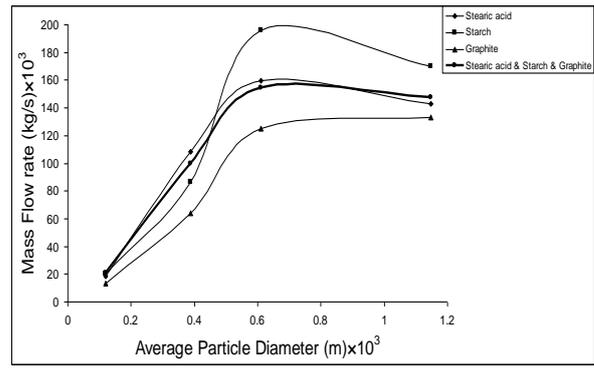
Fig.8. Effect Particles Sizes on Flow With Blends (Stearic Acid & Starch & Graphite)
