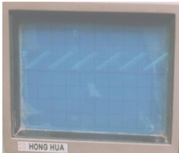
Saw-tooth Waveform, Frequency =125 kHz
