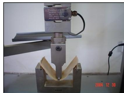
**Fig.4** Bending test of socket
