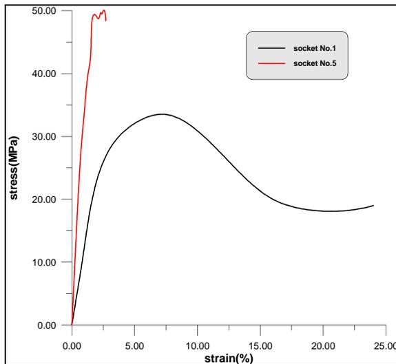
Fig.8 tensile test for socket No.1&5
