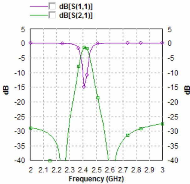
Fig. 6. The Return Loss and Transmission Response of the Dual-Band Microstrip 1<sup>st</sup> Iteration Bandpass Filter.
