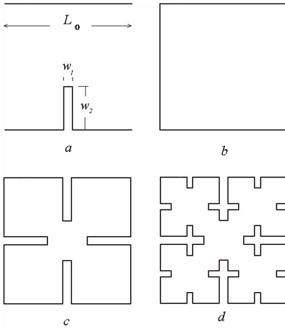
Fig. 1. The Generation Process of the Minkowski-like Prefractal Structure. (a) The Generator. (b) The Square Ring Resonator. (c) The 1<sup>st</sup> Iteration, and (d) The 2<sup>nd</sup> Iteration.
