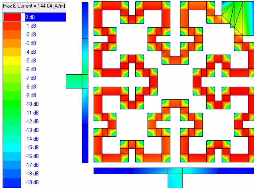
Fig. 8. Current Density Distribution at the Surface of the 2<sup>nd</sup> Iteration Microstrip Bandpass Filter Simulated at 2.4 GHz Resonance Frequency.
