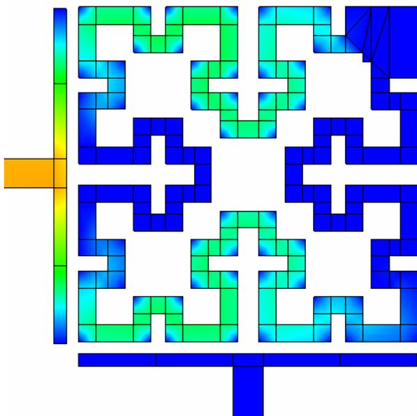
Fig. 9. Current Density Distribution at the Surface of the 2<sup>nd</sup> itEration Microstrip Bandpass Filter Simulated at a Frequency of 2.3 GHz.
