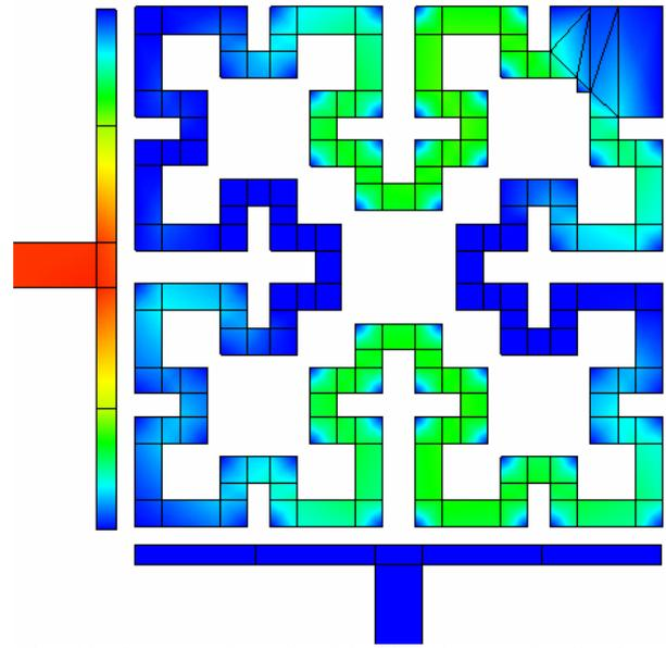
Fig. 10. Current Density Distribution at the Surface of the 2<sup>nd</sup> Iteration Microstrip Bandpass Filter Simulated at a Frequency of 2.5 GHz.
