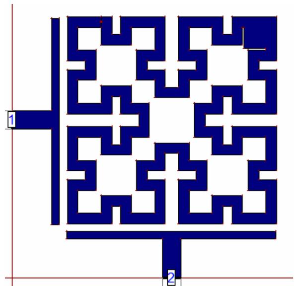
Fig. 4. The Layout of the Dual-Mode Microstrip Bandpass Filter Base on the 2<sup>nd</sup> Iteration.
