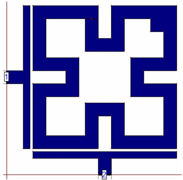
Fig. 3. The layout of the Dual-Mode Microstrip bandpass Fiber Base on the 1<sup>st</sup> Iteration.
