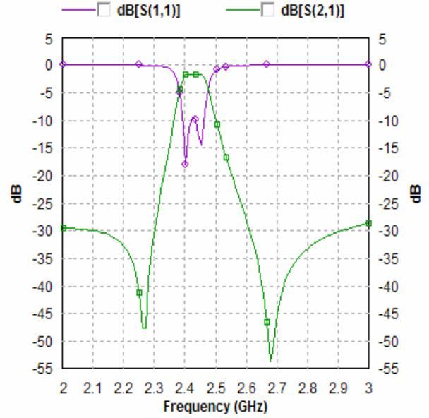
Fig. 7. The Return Loss and Transmission Response of the Dual-Band Microstrip 2<sup>nd</sup> Iteration Bandpass Filter.
