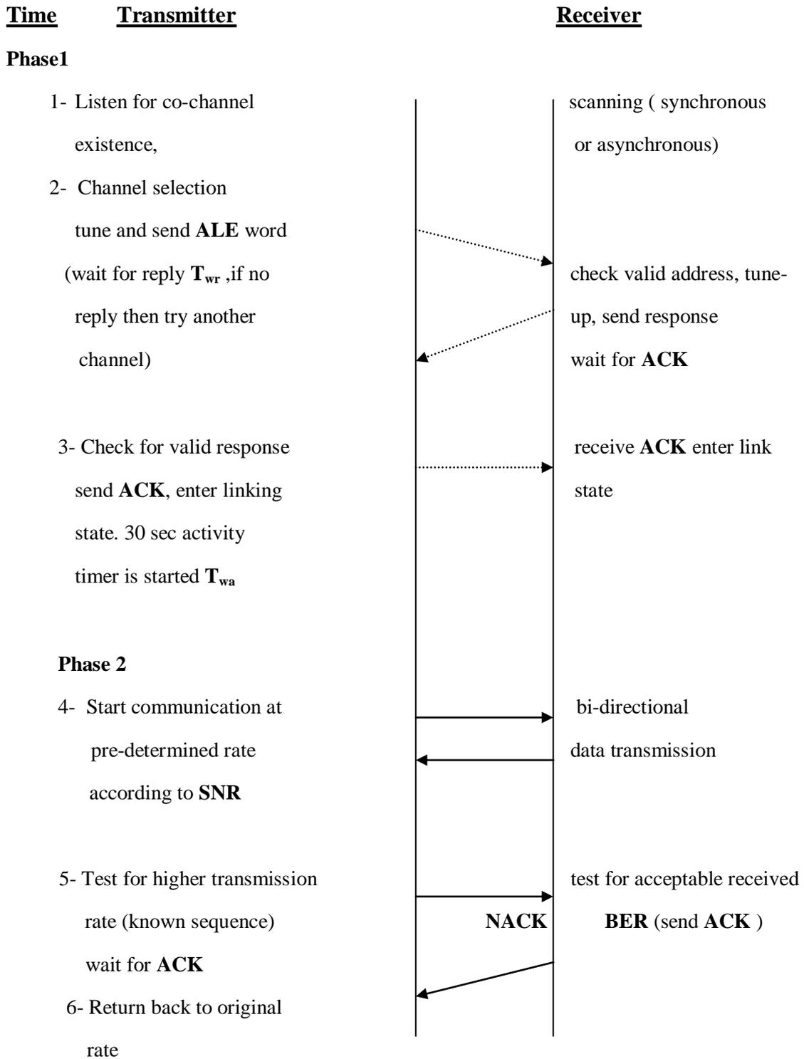
Fig. 3. Adaptation Algorithm for Point to Point.
