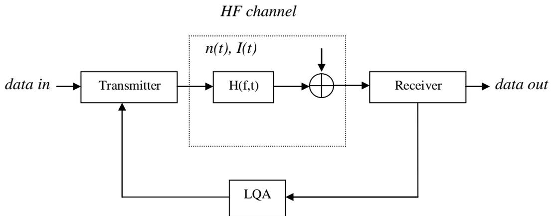
Fig. 1. Block Diagram of HF Radio Link.
