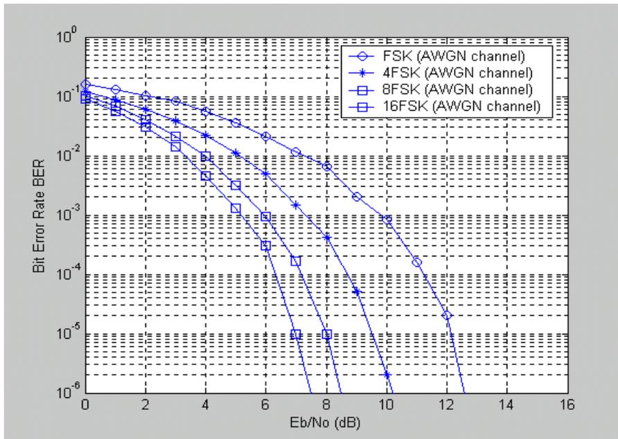
Fig. 7. MFSK Performance Over AWGN Channel (Simulated).
