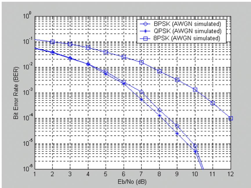
Fig. 8. MPSK Performance Over AWGN Channel (Simulated).
