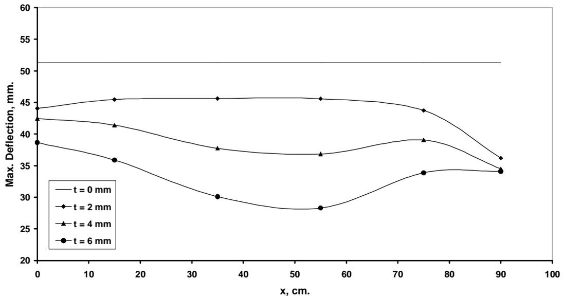
Fig (16) Effect of using two parallel ribs on the maximum deflection for the third case of the design constraints
