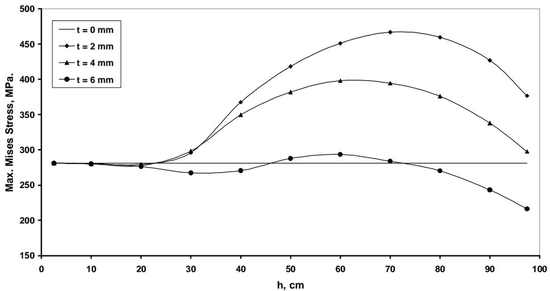
Fig (17) Effect of using one longitudinal rib on one side parallel to the free edge for the third case of the design constraints on the maximum stress
