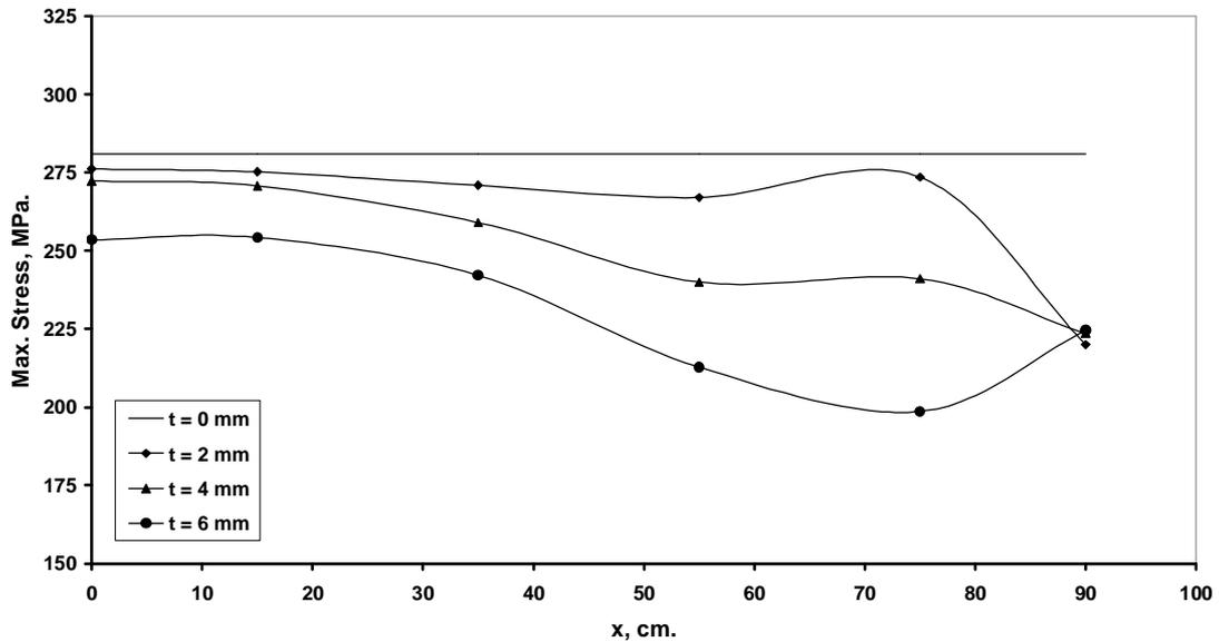
Fig (15) Effect of using two parallel ribs on the maximum stress for the third case of the design constraints
