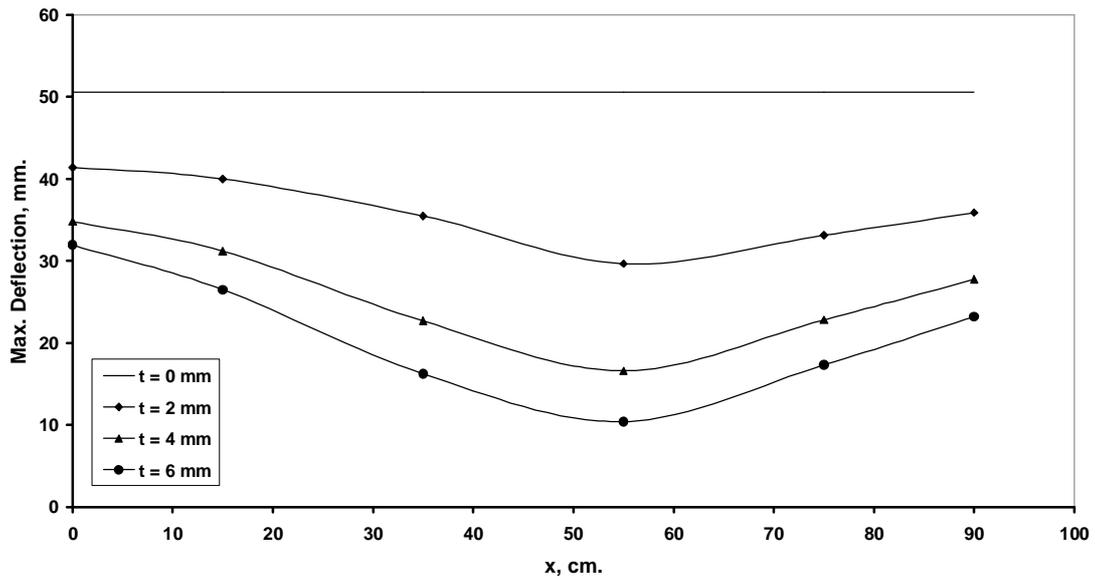
Fig (14) Effect of using two parallel ribs on the maximum deflection for the second case of the design constraints
