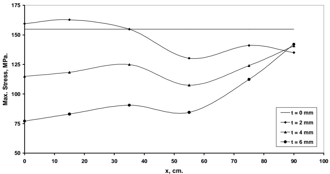
Fig (11) Effect of using two parallel ribs on the maximum stress for the first case of the design constraints
