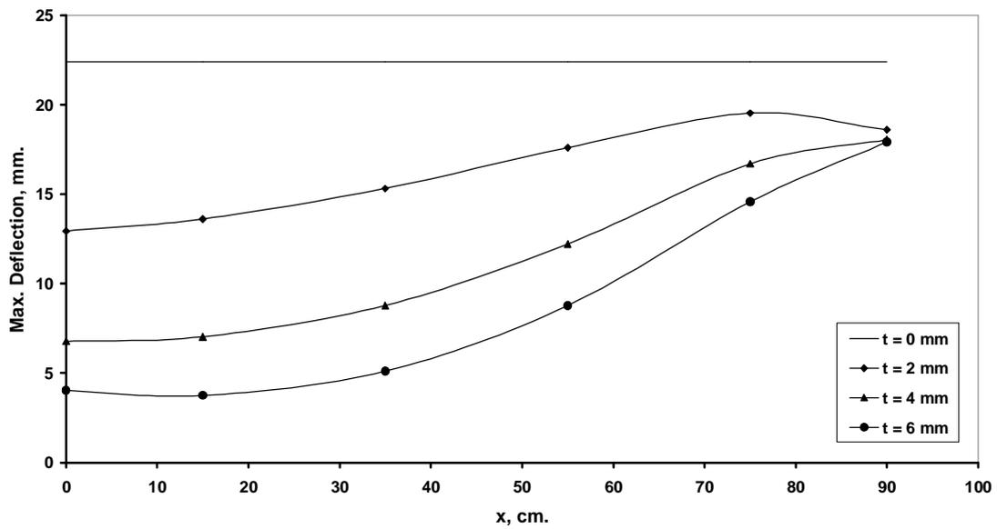
Fig (12) Effect of using two parallel ribs on the maximum deflection for the first case of the design constraints
