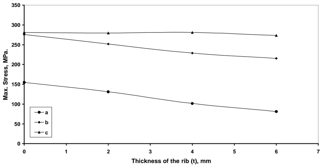
Fig (9) Effect of using one longitudinal rib on two sides on the maximum stress
