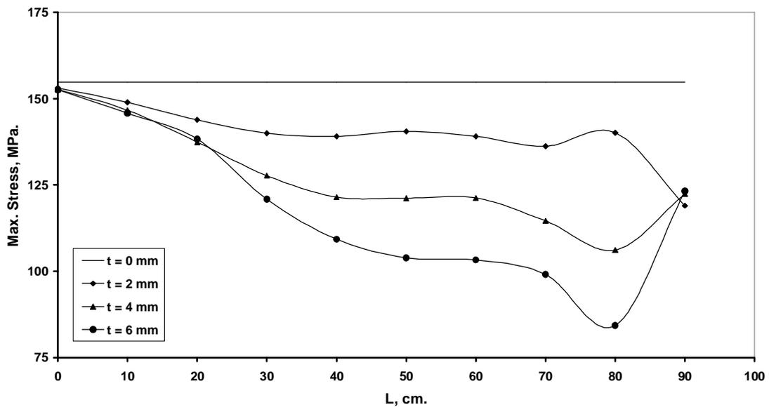
Fig (21) Effect of using one square rib on two sides on the maximum stress for the first case of the design constraints
