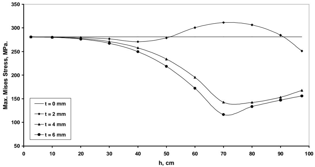
Fig (18) Effect of using one longitudinal rib on two sides parallel to the free edge for the third case of the design constraints on the maximum stress
