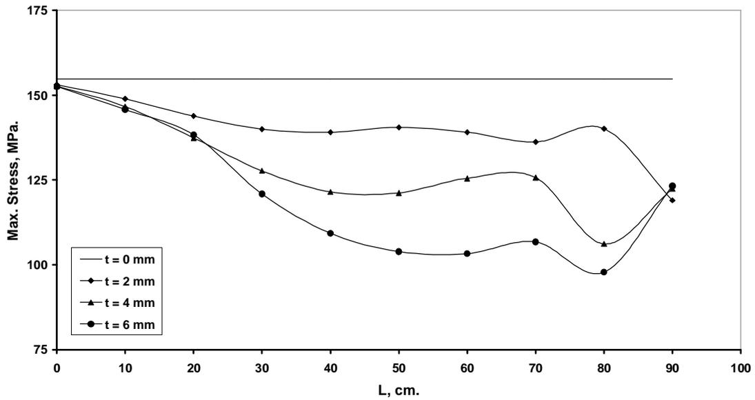
Fig (20) Effect of using one square rib on one side on the maximum stress for the first case of the design constraints
