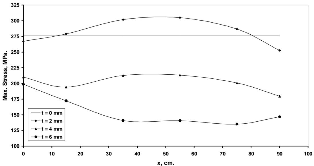
Fig (13) Effect of using two parallel ribs on the maximum stress for the second case of the design constraints
