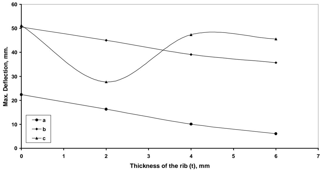
Fig (10) Effect of using one longitudinal rib on one or two sides on the maximum deflection
