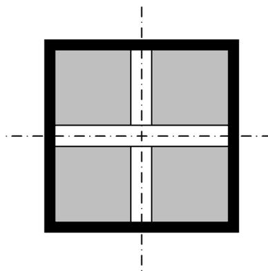
Fig.(7) Two perpendicular longitudinal ribs
