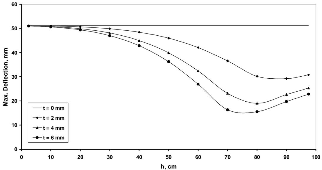
Fig (19) Effect of using one longitudinal rib on one side parallel to the free edge for the third case of the design constraints on the maximum deflection
