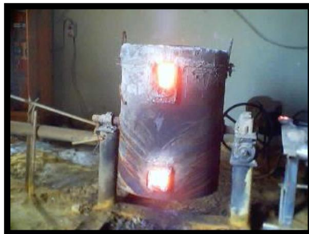
Figure (2) A crucible gas furnace which used in this work
