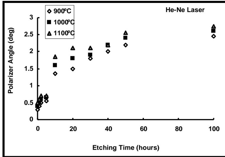
Fig. (3): Polarizer angle vs. etching time for samples fired to (900, 1000, 1100)°C using the He-Ne laser as a light source
