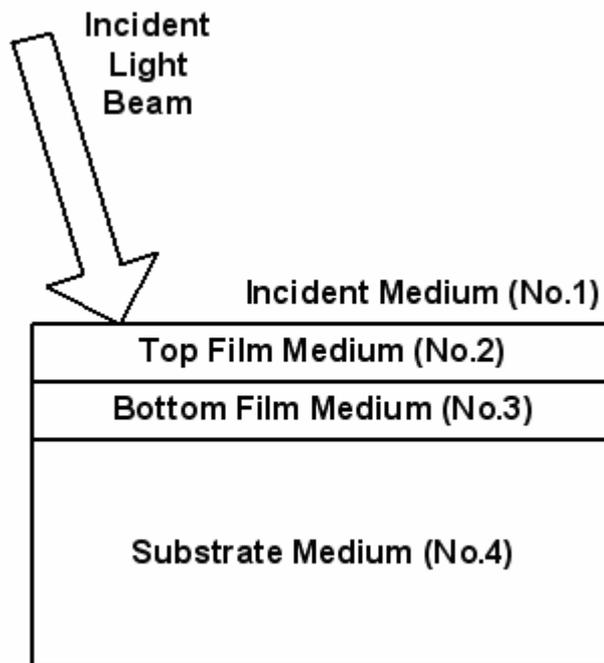
Fig. (2): The model of two-films system considered in this work
