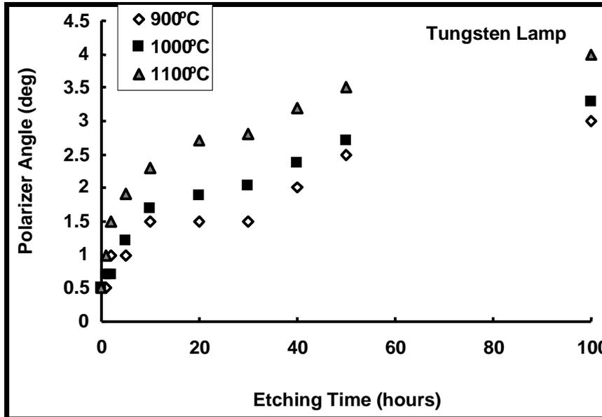
Fig. (5): Polarizer angle vs. etching time for samples fired to (900, 1000, 1100)°C using the tungsten halogen lamp as a light source
