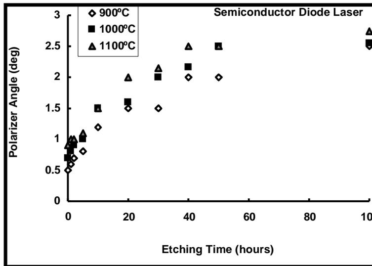
Fig. (4): Polarizer angle vs. etching time for samples fired to (900, 1000, 1100)°C using the semiconductor diode laser as a light source
