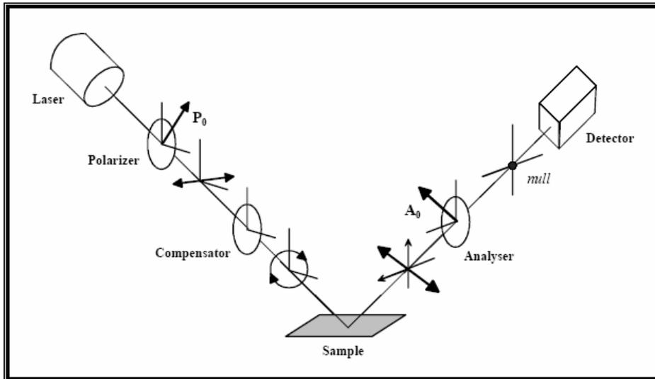
Fig. (1): A schematic diagram of a null-calibration ellipsometer
