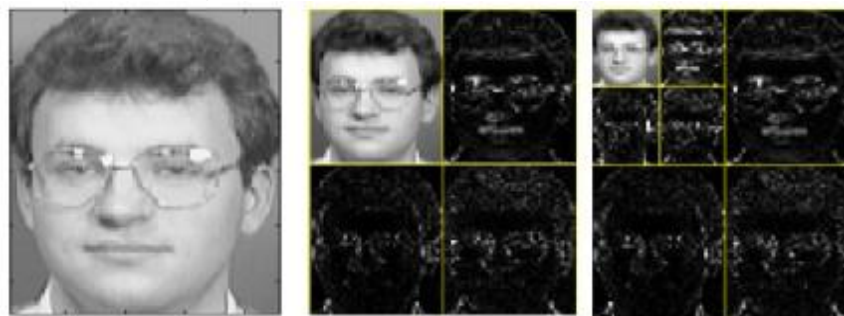
Figure (3) a structure of 3-level 2D-DWT
