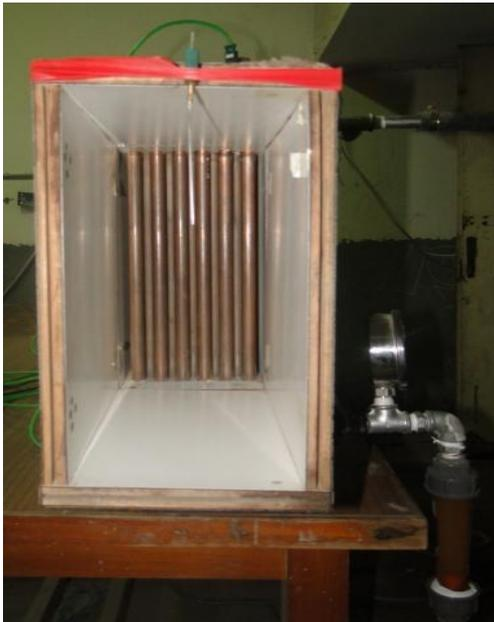
Fig. 6. Plain Tube Heat Exchanger.
