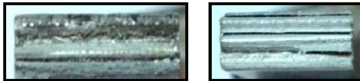
Figure (4) Fracture surfaces showing theseparatingareabetween Stir zone and the base metal
