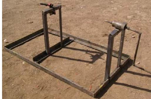
**Fig. 4:** A basic winding machine
