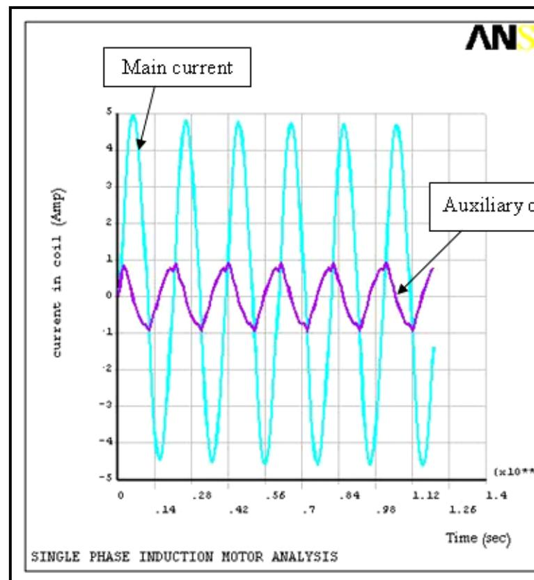
Fig (4) Starting main and auxiliary current versus time at
