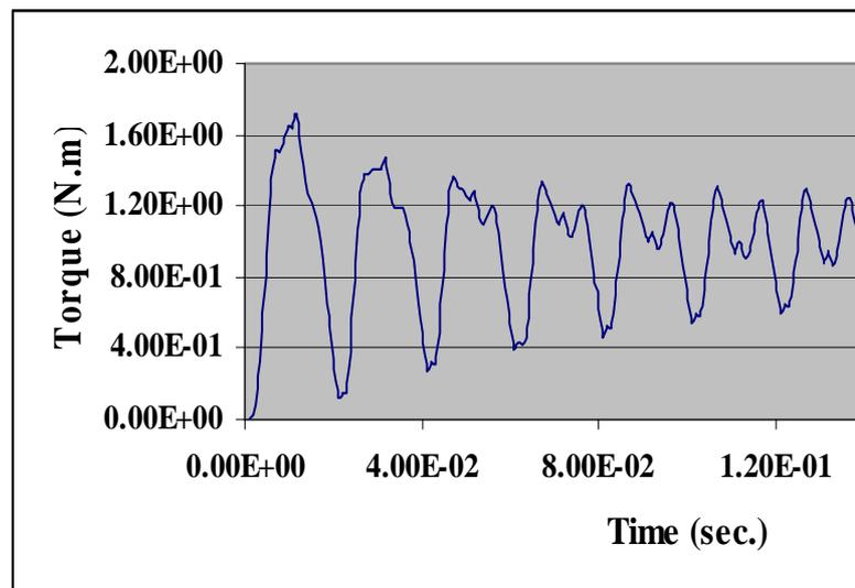
Fig. (10) the variation of starting torque with time at locked rotor condition
