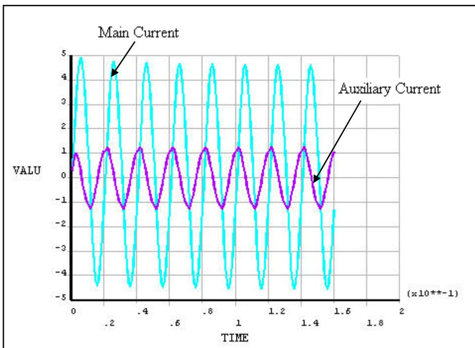
Fig (9) The variation of starting currents with time at locked-rotor condition at  $12 \mu\text{F}$
