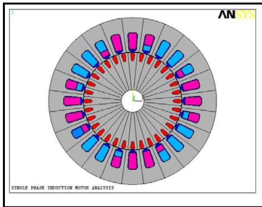
Fig.1 Model of the 2-D SPIM cross section
