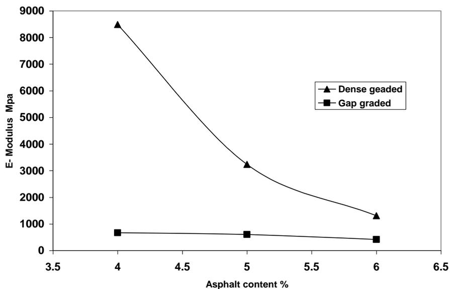
Figure (4) Modulus of Asphalt Concrete
