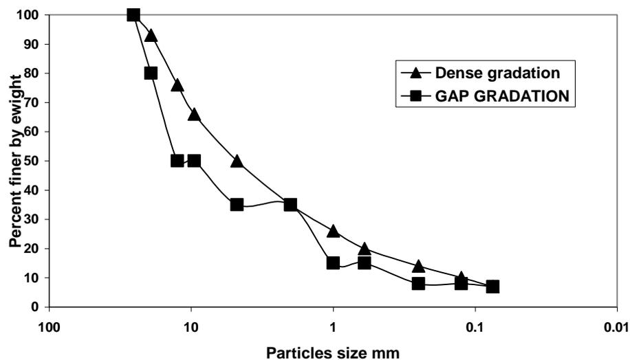
**Figure (1) Grain Size Distribution of the Design Mixes**
