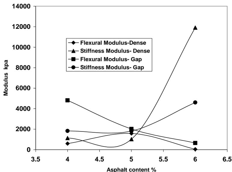
Figure (5) Modulus of Asphalt Concrete
