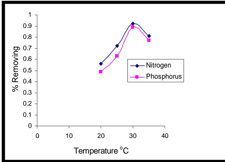
Figure (3) Removing percentage of total nitrogen and total phosphorus from wastewater by microalgae at different temperatures for 2 days
