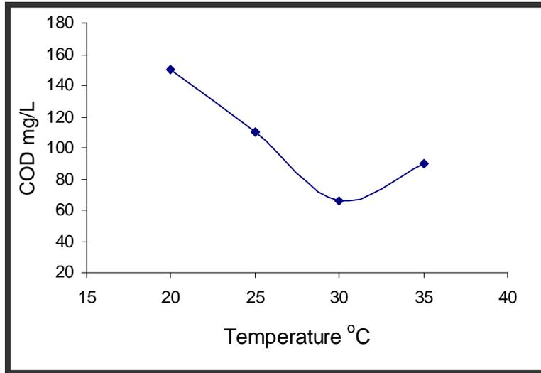
Figure (1) Effect of different temperatures on COD(original concentration was 560 mg/l as COD)
