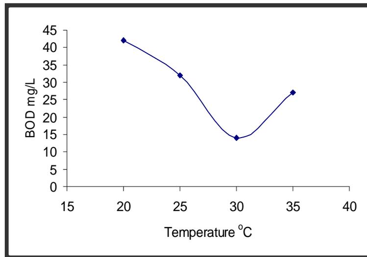
Figure (2) Effect of different temperatures on BOD (original concentration was 135 mg/l as BOD)
