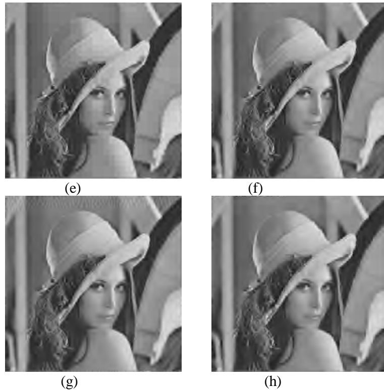
Figure (5) The restored version of the image «Lena», compressed to 0.0625 bpp using two-dimensional algorithm MECT bit wavelet-based structures: a – B_F^9 (26.51 dB); b – H_F^9 (25.09 dB); c – B_F^1 H_F^8 (25.29 dB); d – B_F^2 H_F^7 (25.89 dB); e – B_F^3 H_F^6 (26.42 dB); f – B_F^4 H_F^5 (26.49 dB); g – B_F^5 H_F^4 (26.41 dB); h – H_F^1 B_F^3 H_F^5 (26.31 dB)
