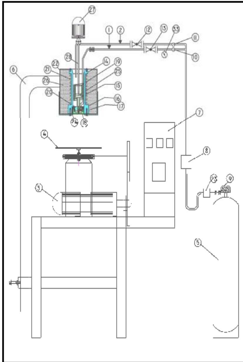
**Figure (3)** 1. N<sub>2</sub> Gas to nozzle, 2. N<sub>2</sub> Gas to furnace, 3. Gearbox, 4. Rotating substrate, 5. N<sub>2</sub> Cylinder, 6. Furnace holder, 7. Control panel, 8. Dryer, 9. Regulator, 10. Flowmeter, 11. Flowmeter, 12. Valve, 13. Valve, 14. Furnace, 15. Crucible, 16. Nozzle, 17. Lower flange, 18. Plate, 19. Coil, 20. Upper flange, 21. Heater, 22. Galv-plate, 23. Oil trap, 24. Thermocouple, 25. Blade, 26. Kaol, 27. Mixer, 28. Shaf
