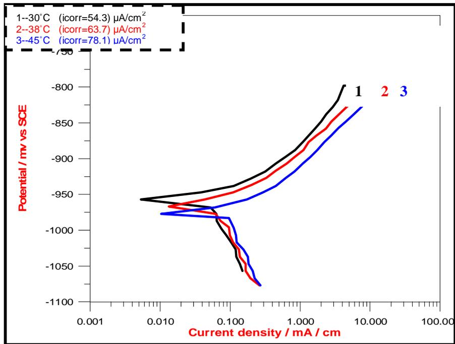
Figure (8) Effect of solution temperature on icorr of 10wt% atomized AMC<sub>5</sub> sample in 3.5% NaCl solution.
