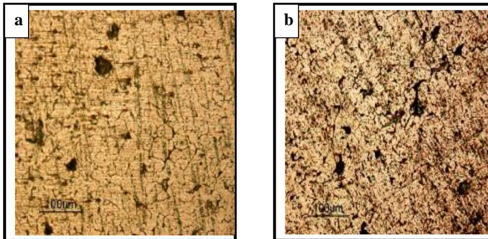
Figure (9): Photographs of (a) Atomized samples before corrosion (200x).
