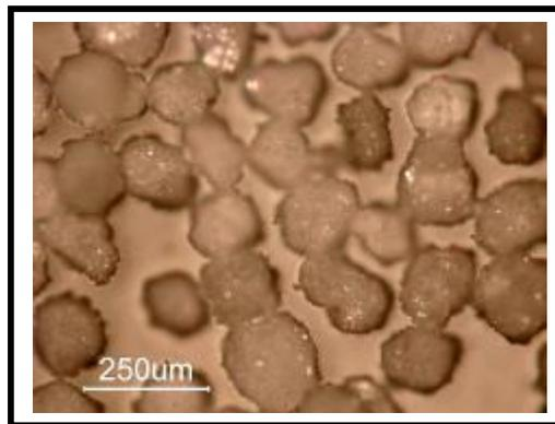
Figure (1) An optical micrograph of The Al<sub>2</sub>O<sub>3</sub> powder (380x)
