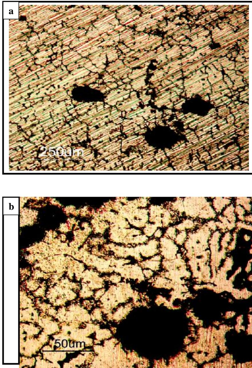
**Figure (10) Photographs of ((a) Atomized AMC<sub>s</sub> samples before corrosion (200x) (b) Atomized AMC<sub>s</sub> samples after corrosion (500x) in 3.5% NaCl solution.**
