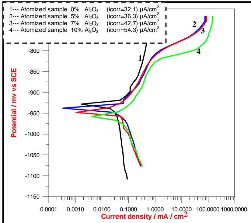
Figure (7) Effect of Al<sub>2</sub>O<sub>3</sub> addition on i<sub>corr</sub> of AMCs samples in 3.5% NaCl solution at temperature 30 °C.
