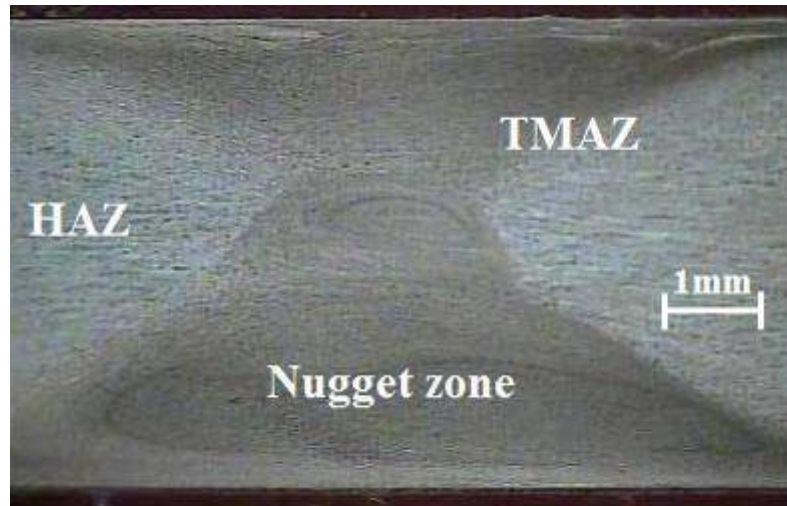
Fig.12 .Macrostructure of specimen welded with 0.5 mm interference and same rotational speed direction
