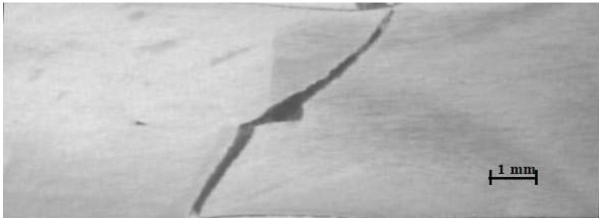
Fig. 11 .Failure of 0.5 mm pin interference specimens
