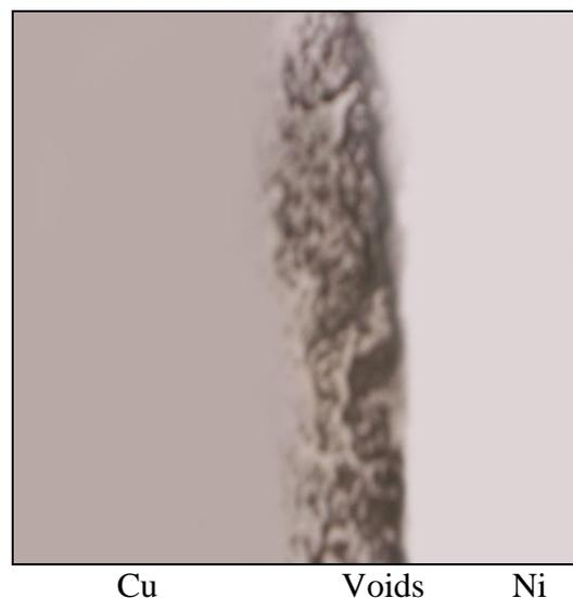
Figure (6) Micrograph of the bonded joints Cu-Ni, Magnification (176X) shows the voids formation in the copper side of the bonded joints at  $T=750\text{ }^{\circ}\text{C}$ , time =30 min, surface roughness=  $0.2\text{ }\mu\text{m}$ , and bonding pressure = $0.353\text{N/mm}^2$
