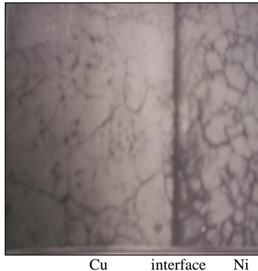
Figure (5) Micrograph of the microstructure for the bonded joints Cu-Ni Magnification (300X), shows the interface between Cu & Ni parts, at  $T=700\text{ }^{\circ}\text{C}$ , time =30 min, surface roughness=  $0.2\text{ }\mu\text{m}$ , and bonding pressure = $0.353\text{N/mm}^2$
