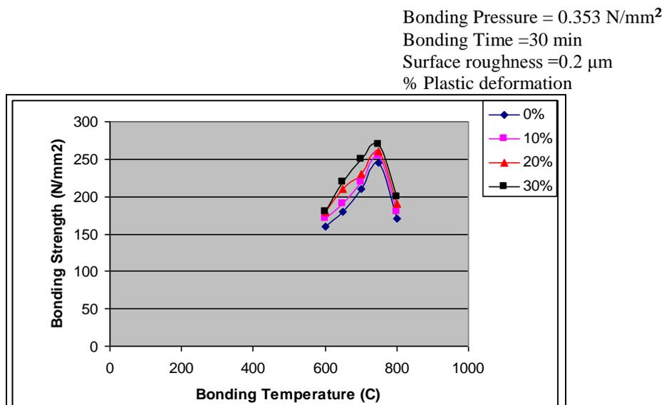
**Figure (1) Bonding temperature vs tensile strength of diffusion bonded joints Cu-Ni for different plastic deformation**
