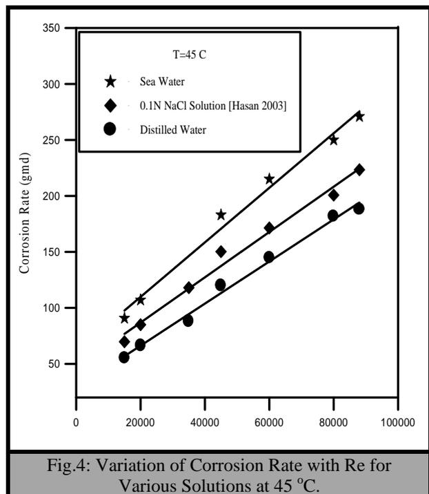
Fig.4: Variation of Corrosion Rate with Re for Various Solutions at 45 °C.
