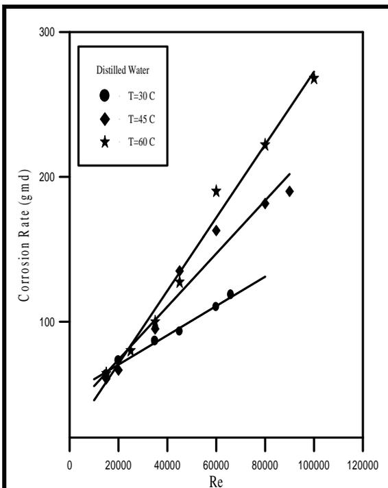
Fig. 6: Effect of Temperature on the Corrosion Rate.
