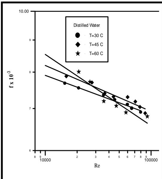
Fig. 2: Variation of friction factor with Re at different temperatures.
