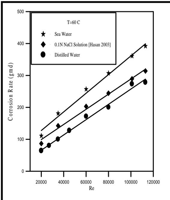
Fig. 5: Variation of Corrosion Rate with Re for Various Solutions at 60 °C.
