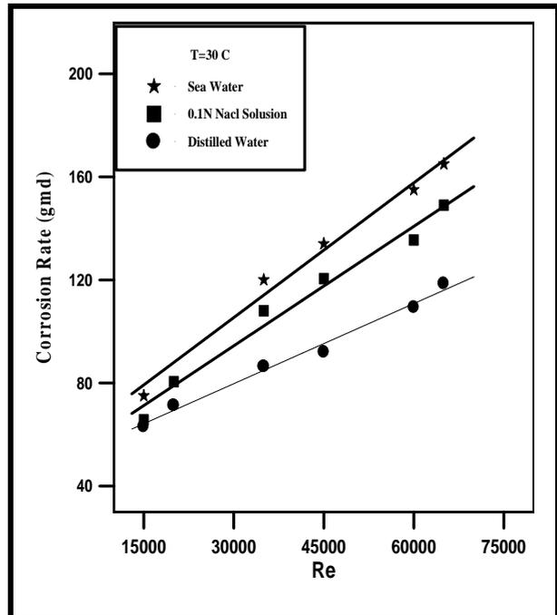
Fig. 3: Variation of Corrosion Rate with Re for Various Solutions at 30 °C.
