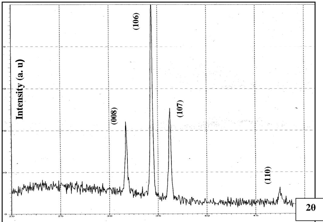
Figure 2: X-ray diffraction pattern (XRD) of ZnS thin film at 723K
