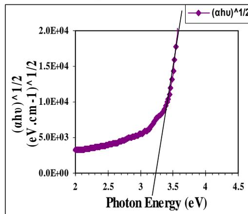
Figure 9-b: The optical energy gap for the indirect allowed transition of ZnS films at substrate temperatures 723K
