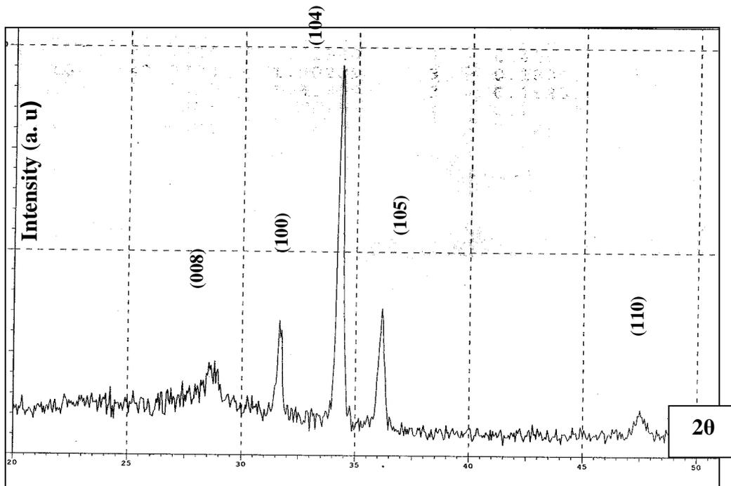
Figure 1: X-ray diffraction pattern XRD of ZnS thin film at 673K
