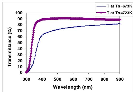
Figure 3: The transmission spectra of ZnS films as a function of wavelength at both substrate temperature of 673K and 723K
