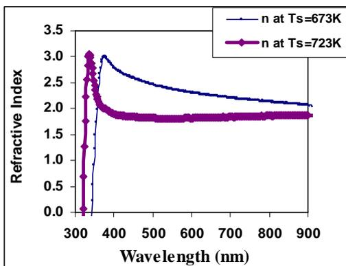
Figure10: The refractive index of ZnS thin films for both substrate temperatures of 673K and 723K
