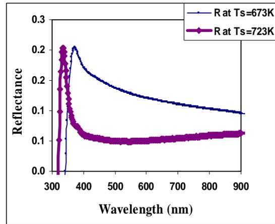
Figure 5: The reflectance spectra of ZnS thin films as a function of the wavelength prepared at both substrate temperatures of 673K and 723K
