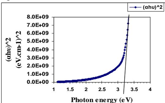
Fig.8-a: The optical energy gap for the direct allowed transition of ZnS thin films at substrate temperatures 673K
