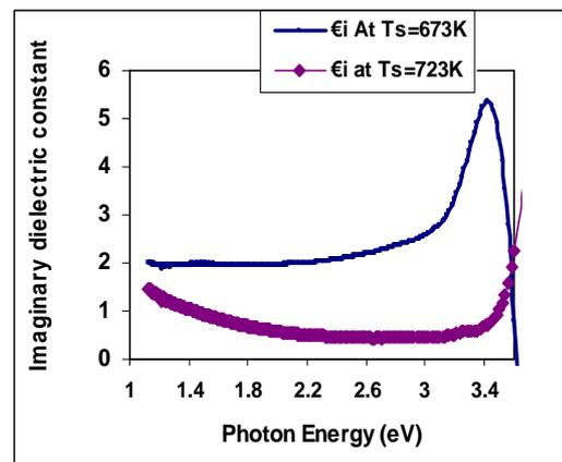
Figure 11: The imaginary parts of dielectric constant for both substrate temperatures of 673K and 723K
