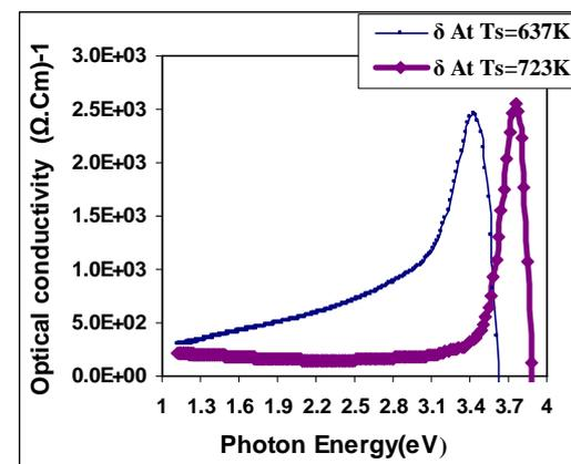
Figure 12: The optical conductivity of ZnS thin films for both substrate temperatures of 673K and 723K
