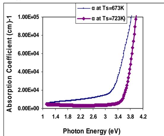
Figure 6: The absorption coefficient of ZnS thin films as a function of wavelength at both substrate temperatures of 673K and 723K
