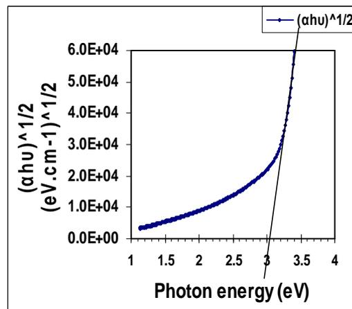
Figure 9-a: The optical energy gap for the indirect allowed transition of ZnS thin films at substrate temperatures 623K
