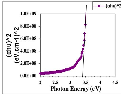
Figure8-b: The optical energy gap for the direct allowed transition of ZnS thin films at substrate temperatures 723K
