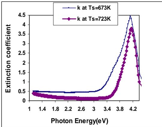
Figure 7: The extinction coefficient of ZnS thin films as a function to the photon energy at both substrate temperatures of 673K and 723K
