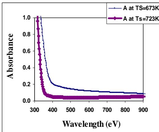
Figure 4: The absorption spectra of ZnS thin films as a function of wavelength prepared at both substrate temperature of 673K and 723K
