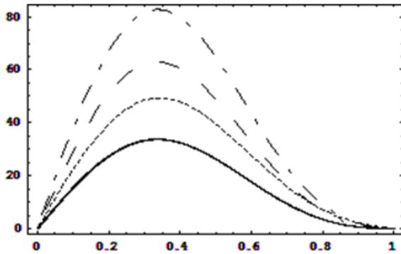
Fig 6 : Velocity profile for  $M = 0.001, 1, 2, 4$
