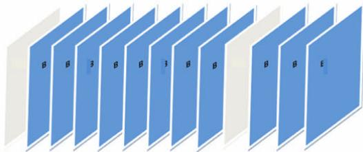
**Figure 4: Illustration above how atypical sequence with I-, B-, and p frame may look. Note that a p-frame may only reference a preceding I-or P-frame while a B-frame may both preceding and succeeding I-and P-frames.**
