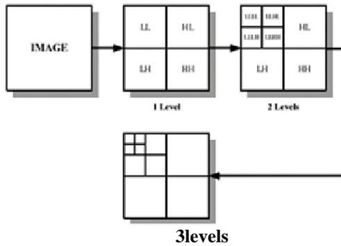
Figure 1: Two dimensional wavelet Transform
