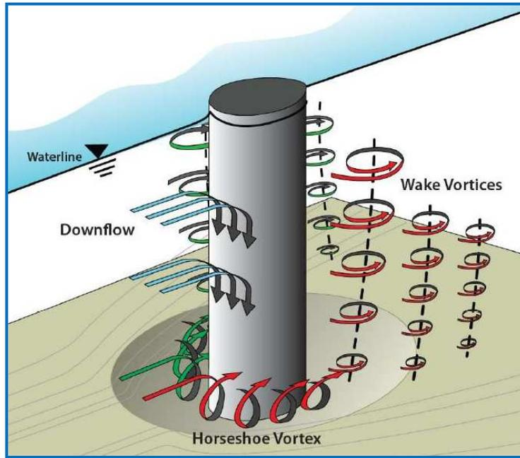
(Fig.1) Schematic representation of scour around bridge pier [7]
