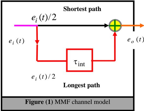
The transmitted power is assumed to be equally distributed among these two modes. Let  $e_i(t)$  is the signal electric field incident on the input of the fiber. The input electric field of each of the fastest and slowest modes is equal to  $e_i(t)/2$ . If the fiber attenuation is neglected (an assumption which is justified for short link), then field at the fiber end is given by
