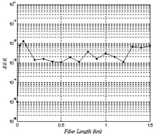
(b) 16-QAM SNR = 13.47dB ( $P_b = -32.25\text{dBm}$ )
