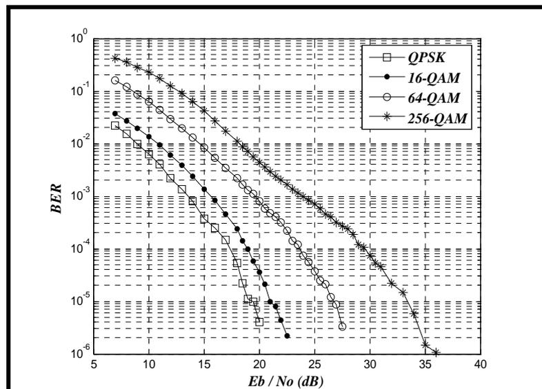
**Figure (10)** BER Performance of OFDM system over MMF channel with ( $L = 1\text{km}$ ).
