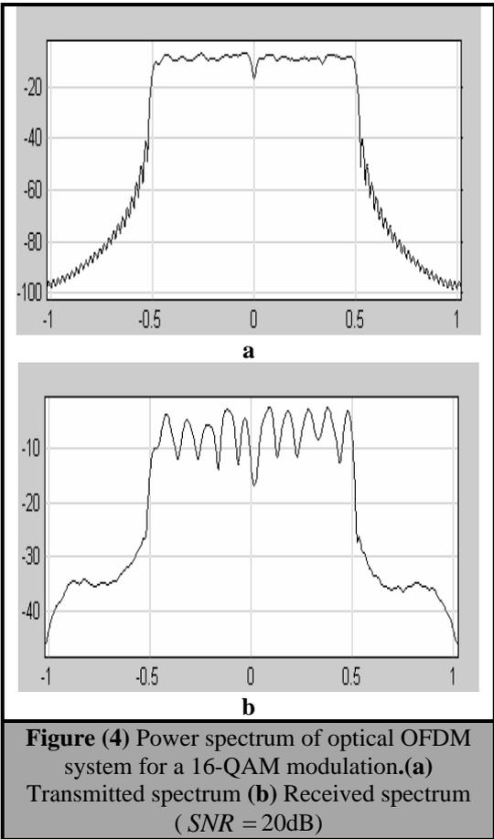
**Figure (4)** Power spectrum of optical OFDM system for a 16-QAM modulation.(a) Transmitted spectrum (b) Received spectrum ( $SNR = 20\text{dB}$ )
