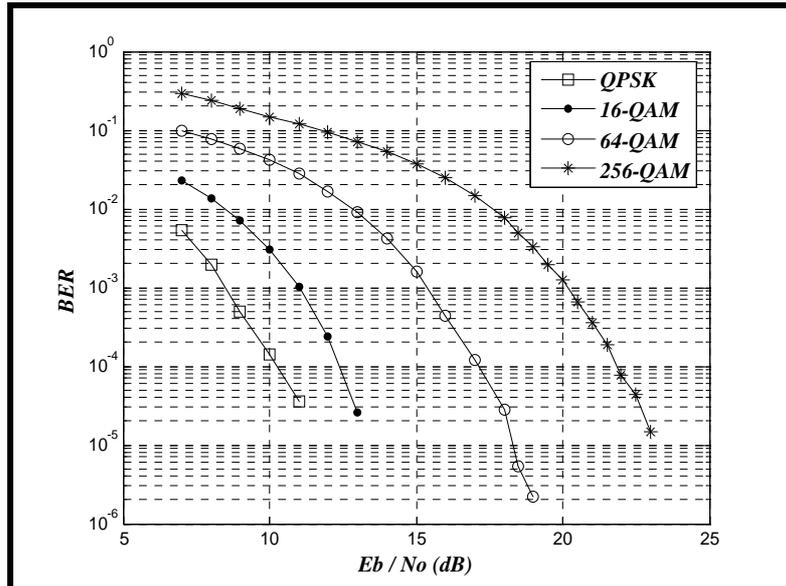
**Figure (9)** BER performance of OFDM system in the absence of fiber dispersion ( $L = 0$ ).
