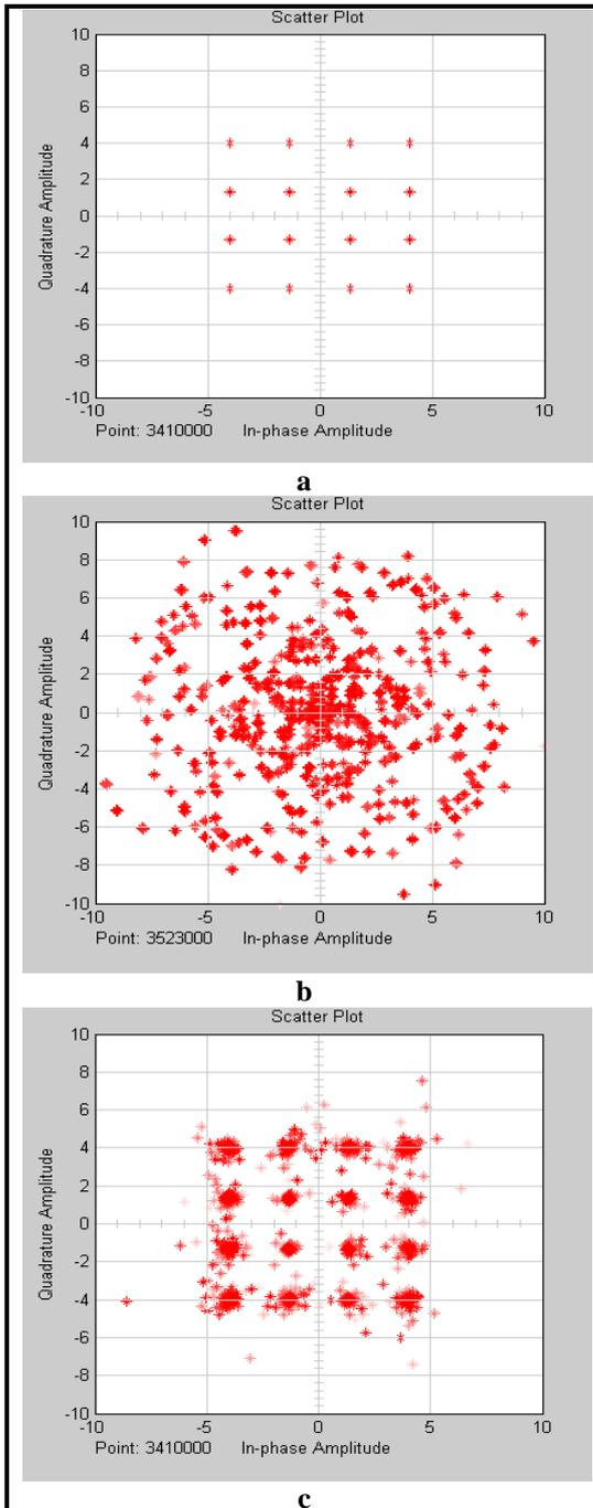
**Figure (3)** Signal constellation diagrams for a 16-QAM optical OFDM system when  $SNR = 20\text{dB}$  (a) In the transmitter (b) In the receiver without channel estimation (c) In the receiver with channel estimation.
