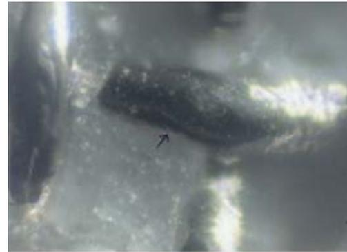
**Fig. (8): Black precipitate at the mesh of the bracket**
