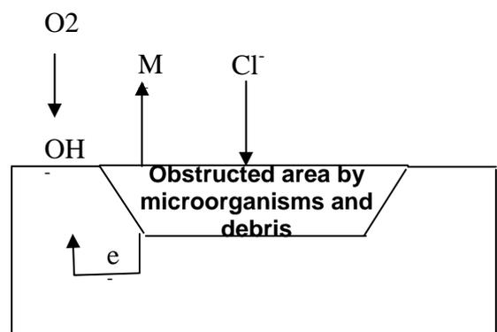
**Fig. (10): Role of micro-organisms in the development of corrosion**
