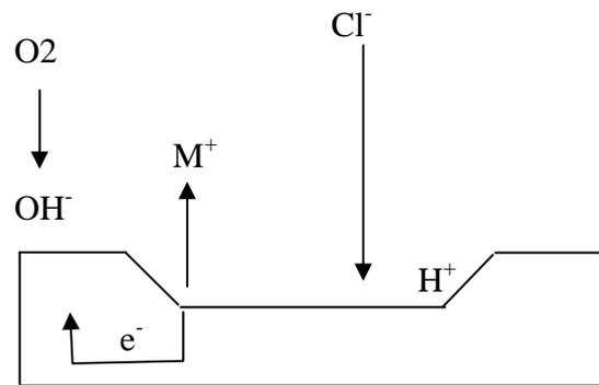
**Fig. (9): Mechanism of pitting corrosion**
