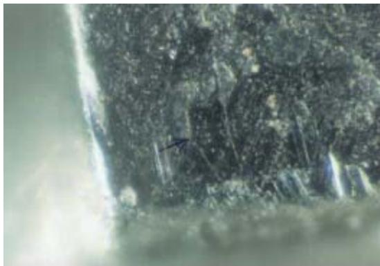
Fig(3): Pitting corrosion at the wing of the bracket
