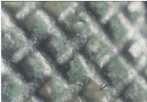
**Fig.(7): Gree and Brown precipitate at the mesh of the bracket**
