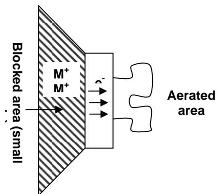
**Fig. (11): Corrosion at the mesh of the bracket**
