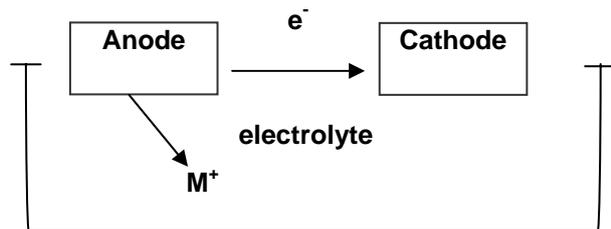
Fig. (1) Electrochemical cell
