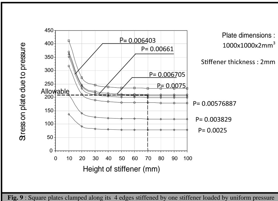
**Fig. 9 :** Square plates clamped along its 4 edges stiffened by one stiffener loaded by uniform pressure
