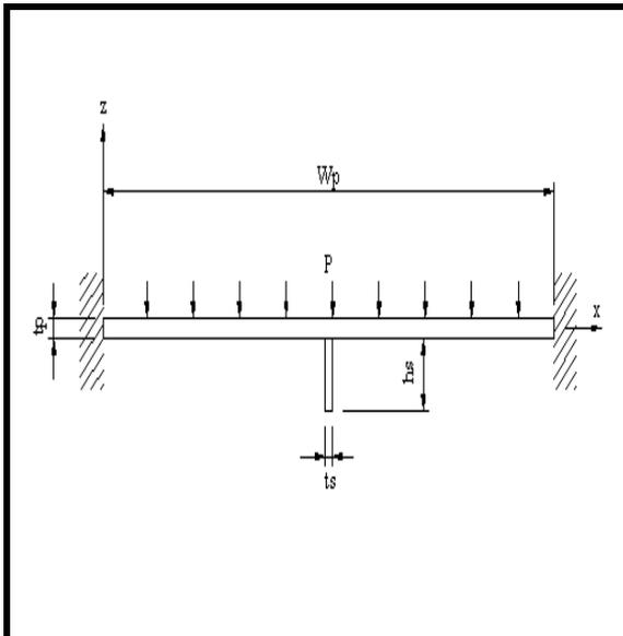
**Fig. 1:** Side view of the model
