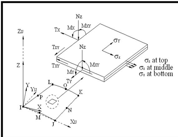
Fig. 4: Shell type 93 element
