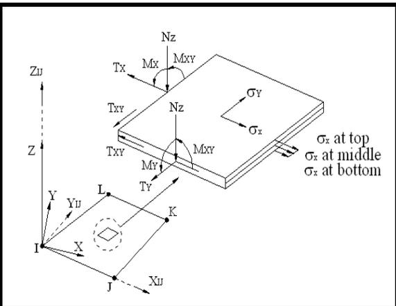
Fig. 5: Shell type 63 element
