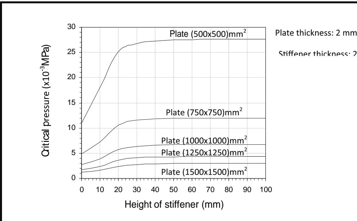
Fig. 11 : Critical curves for square plate clamped along 4 edges
