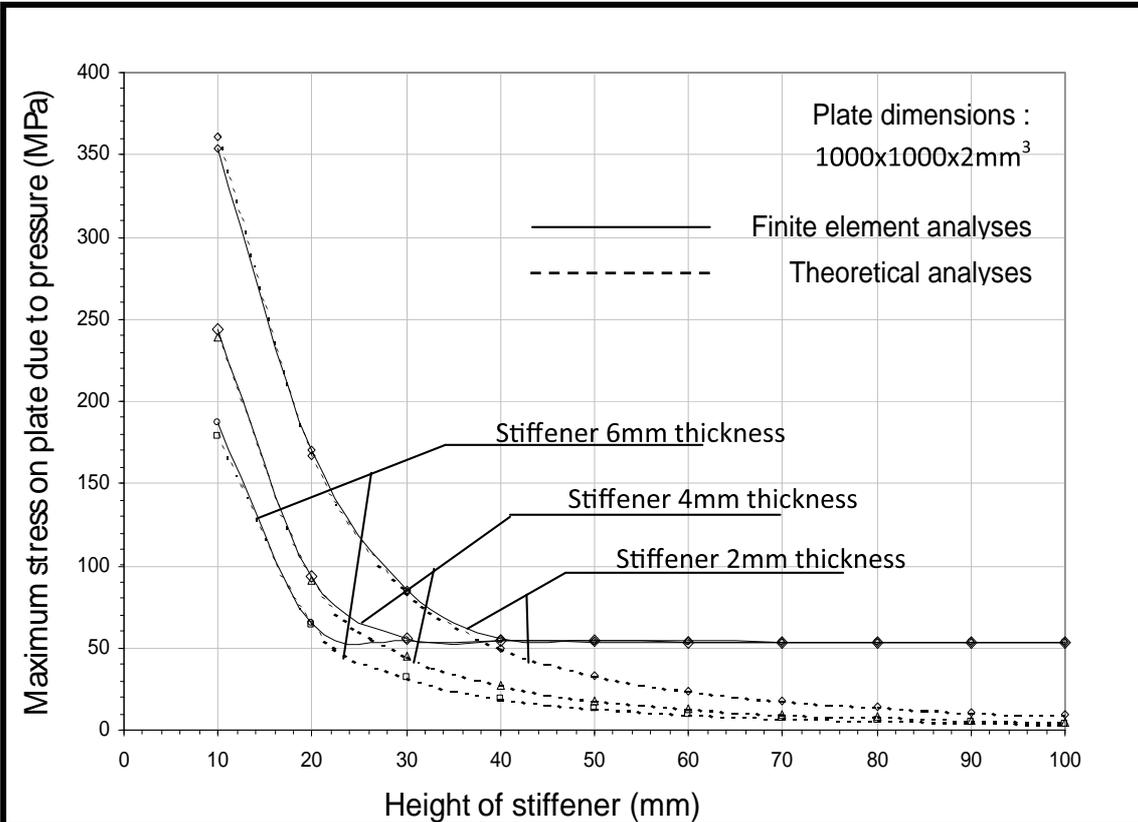
Fig. 10 : Comparison between finite element and theoretical analyses methods to compute maximum stress in stiffened square plate clamped along its 4 edges subjected to uniform pressure
