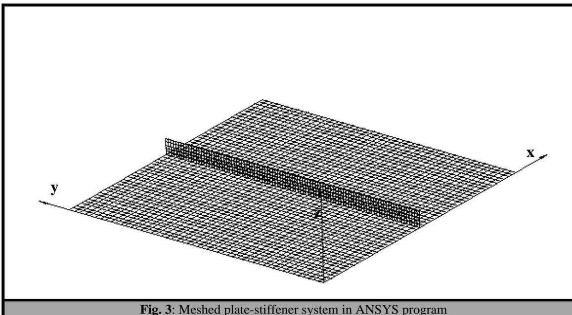
**Fig. 3:** Meshed plate-stiffener system in ANSYS program
