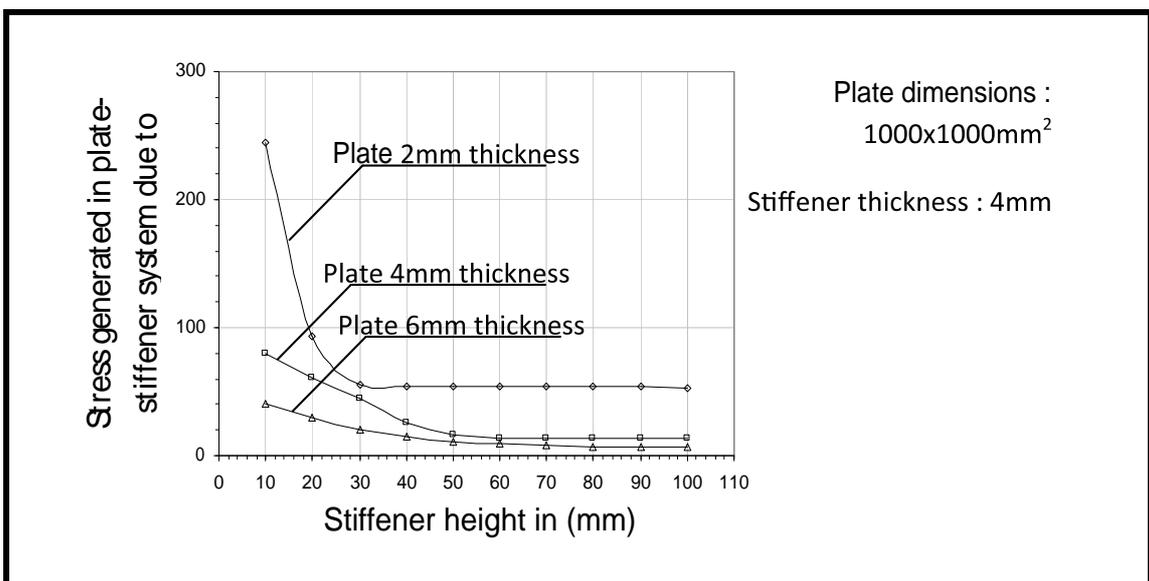
Fig. 7: Effect of plate thickness on stress generated in a square plate having one stiffener and clamped along its 4 edges loaded by pressure
