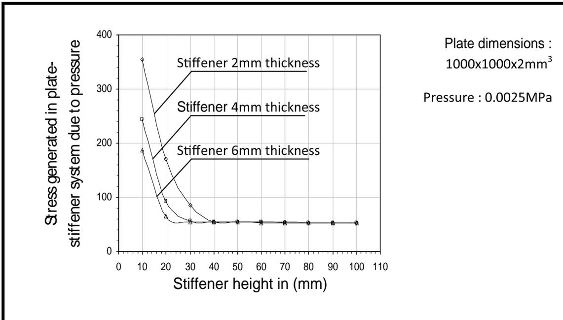
**Fig. 8:** Effect of stiffener thickness on stress generated in a square plate having one stiffener and clamped along its 4 edges loaded by pressure
