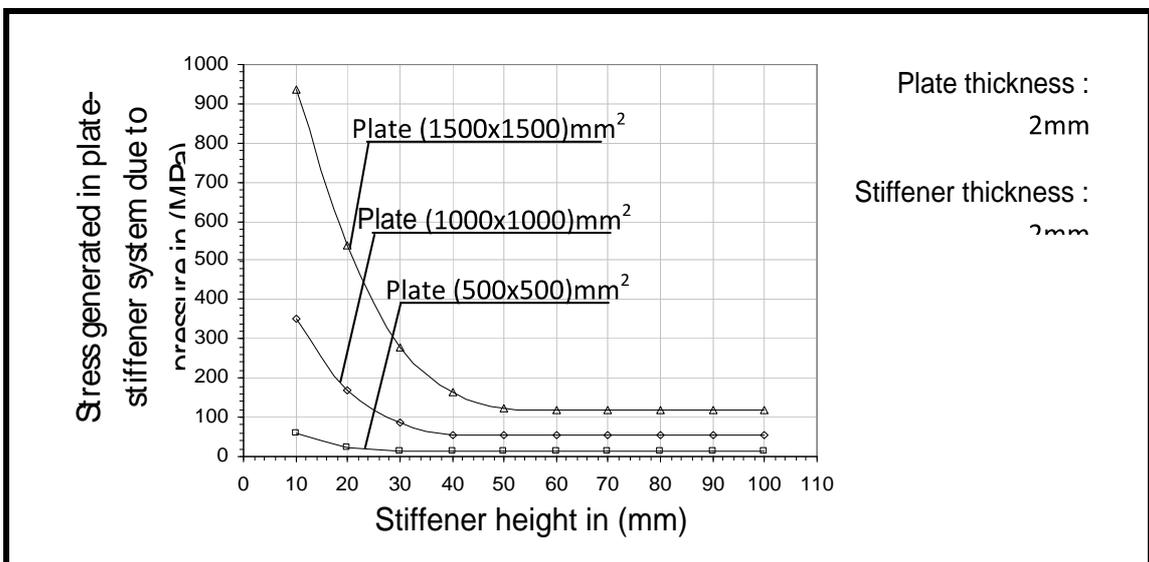
Fig. 6 : Effect of plate dimensions on stress generated in a square plate having one stiffener and clamped along its 4 edges loaded by pressure
