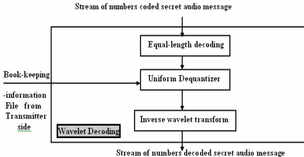
**Fig.(4) Wavelet Decoding**
