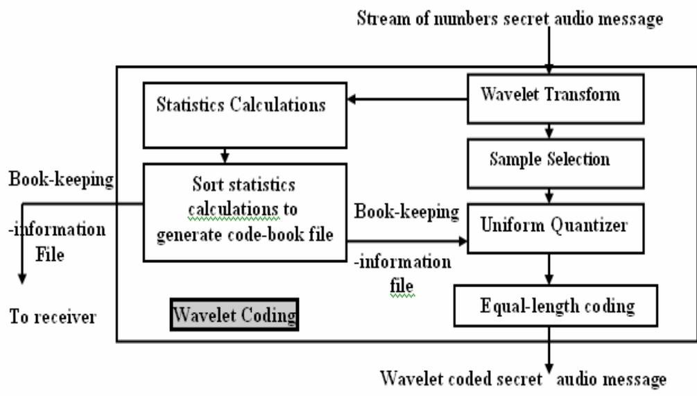
**Fig.(3) Wavelet Coding**
