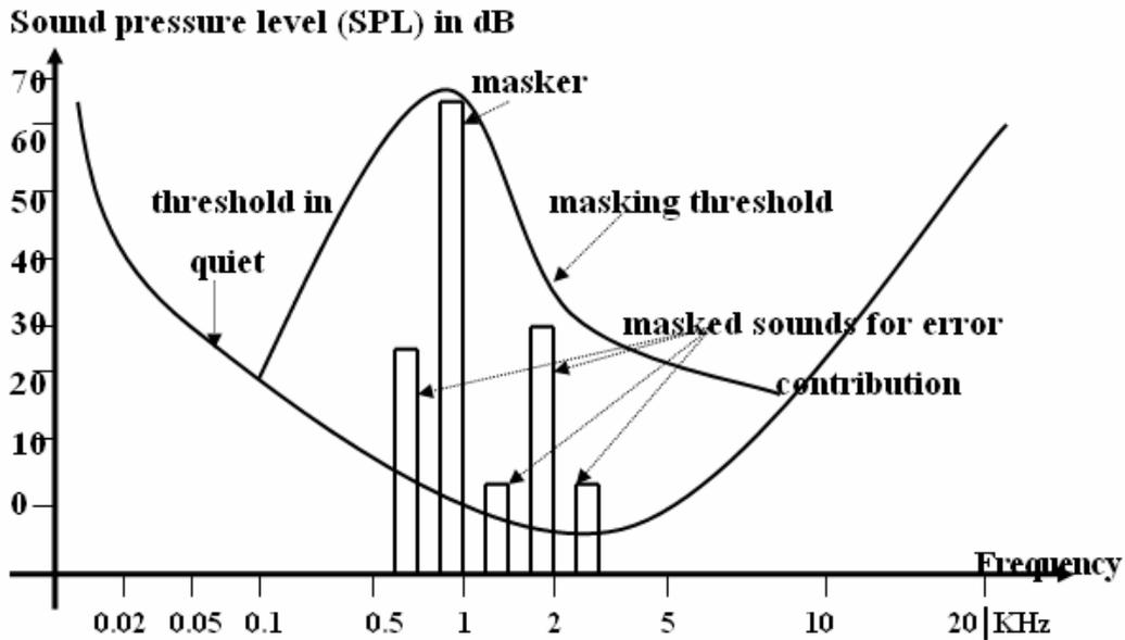
Figure (1) Threshold in quite and masking threshold acoustical events in the closed curve area will not be audible
