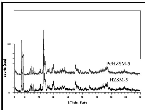
**Fig. 2:** XRD for original HZSM-5 and for Pt/HZSM-5 loaded by impregnation method
