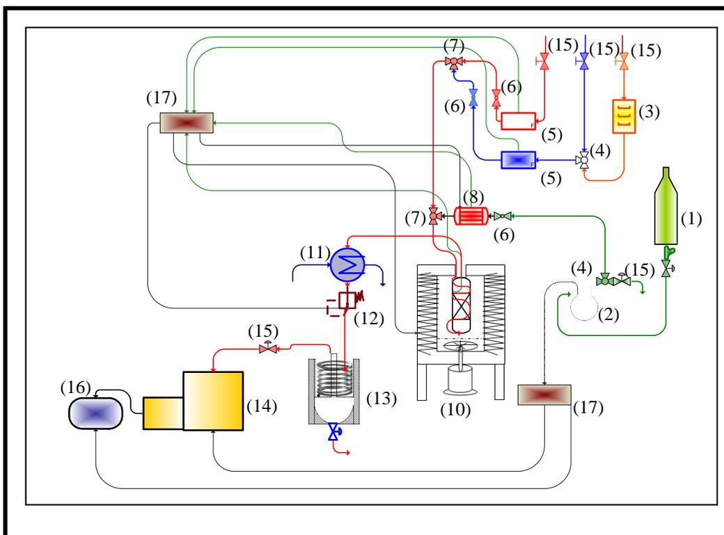
**Fig.1:** schematic flow diagram of catalytic experiment rig,
