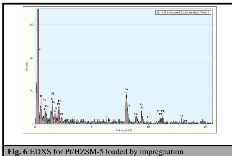
**Fig. 6:**EDXS for Pt/HZSM-5 loaded by impregnation
