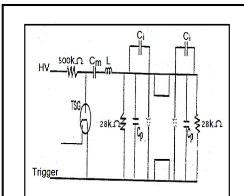
**Fig.(5) Electrical Excitation Circuit with Preionization**
