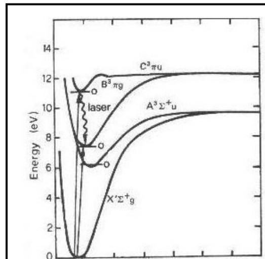
**Fig(1) Energy levels of the N<sub>2</sub> molecule . For simplicity only the lowest vibrational level (v=0) is shown for each electronic state [2].**
