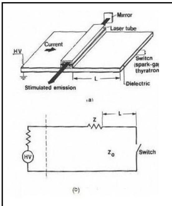
**Fig (2)** (a) Blumlein pulse generator using a flat transmission line. The discharge channel may typically be  $2 \times 0.5$  cm, the large dimension being along the discharge direction. (b) Transmission line analog of the Blumlein generator above[2].
