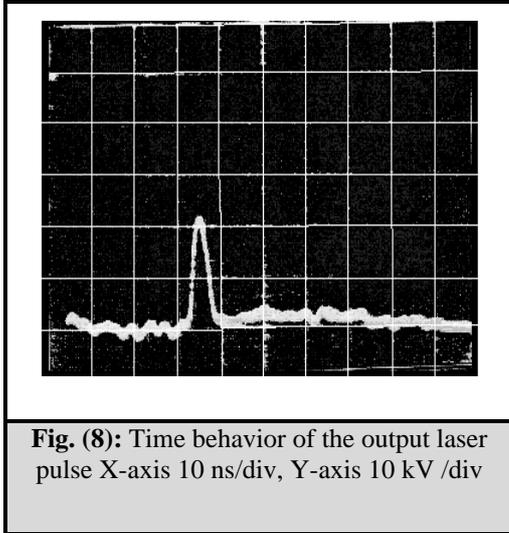
**Fig. (8):** Time behavior of the output laser pulse X-axis 10 ns/div, Y-axis 10 kV /div
