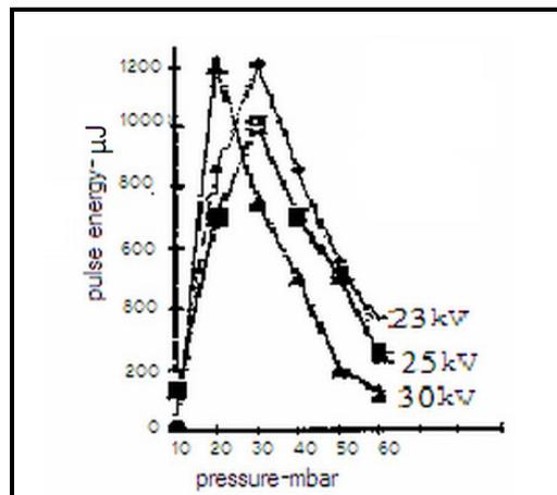
**Fig.(6) Pulse dependence on pressure for different applied voltage**
