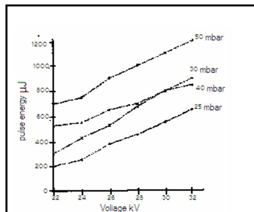
**Fig.(7) Pulse Energy Dependence on Applied voltage for Different Pressures**
