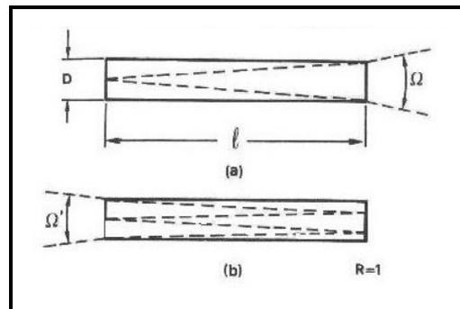
**Fig. (3)** Solid angle of emission in the case of amplified spontaneous emission: (a) active material without any end mirror: (b) active material with one end mirror[2].
