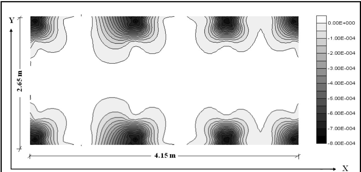
**Figure (6): Horizontal principal tensile strain at the bottom of asphalt layer ( $\epsilon_x$ ) ( $t_1=7.6$  cm and  $t_2=56.6$  cm).**
