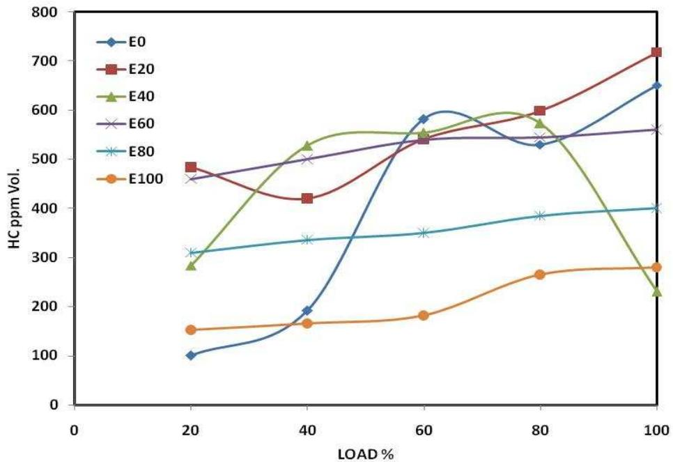
Figure 3. Effect of ethanol blending on the HC emissions at different engine loads.
