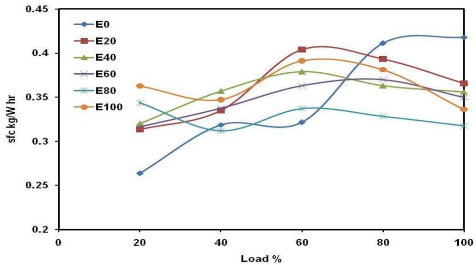
Figure 6. Effect of ethanol blending on the specific fuel consumption at different engine loads.
