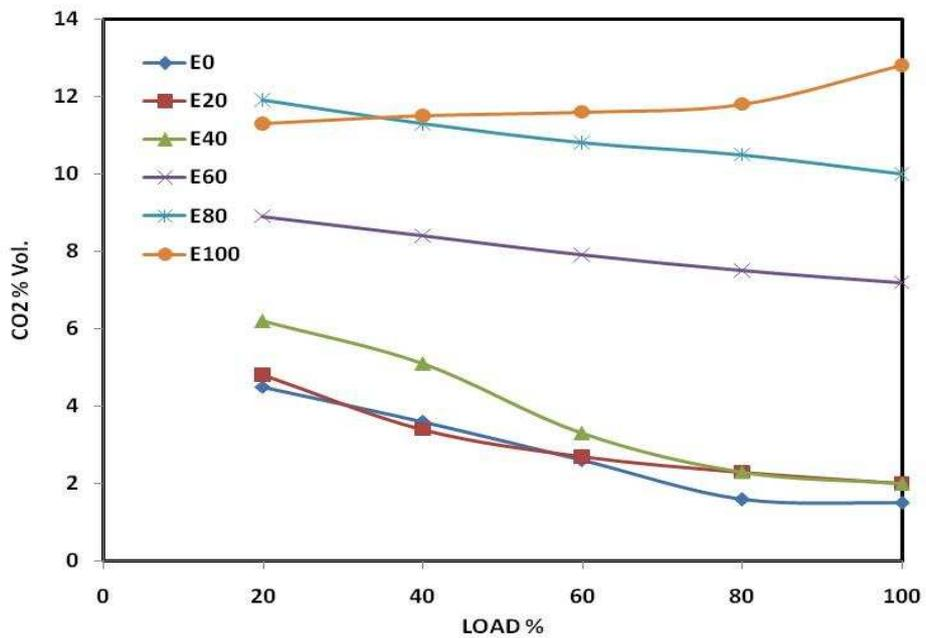
Figure 5. Effect of ethanol blending on the CO<sub>2</sub> emissions at different engine loads.
