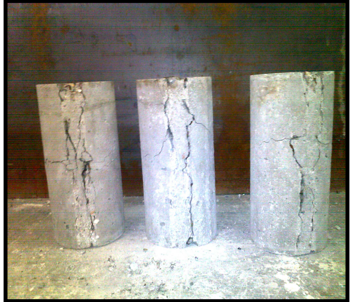
Figure (10) Modes of failure of concrete specimens with fiber content
