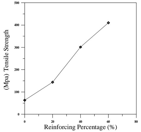
Figure (4): Tensile Strength
