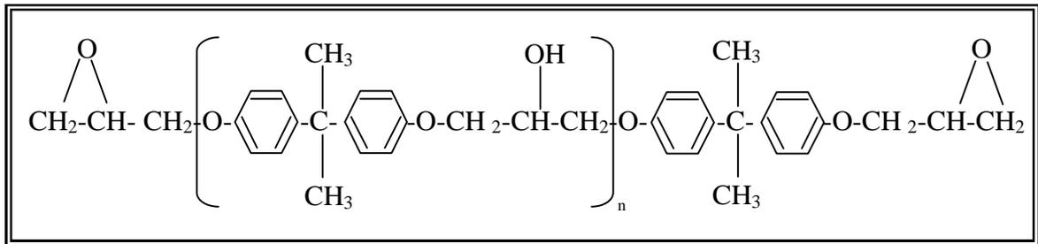
Figure (1): Chemical structure of Araldite resin [Mallick,2007]
